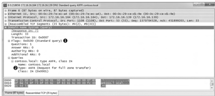
Figure 7-16: DNS full zone transfer request
