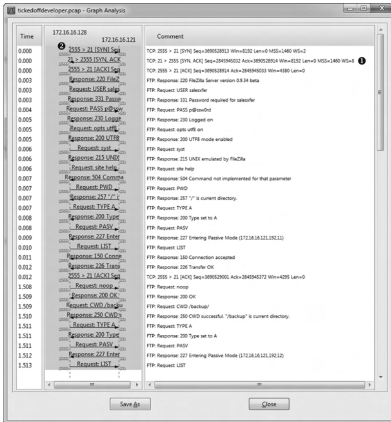
Figure 8-37: The flow graph gives a quick view of the FTP communication.
