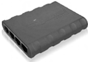
Figure 2-7: A Barracuda nonaggregated tap
