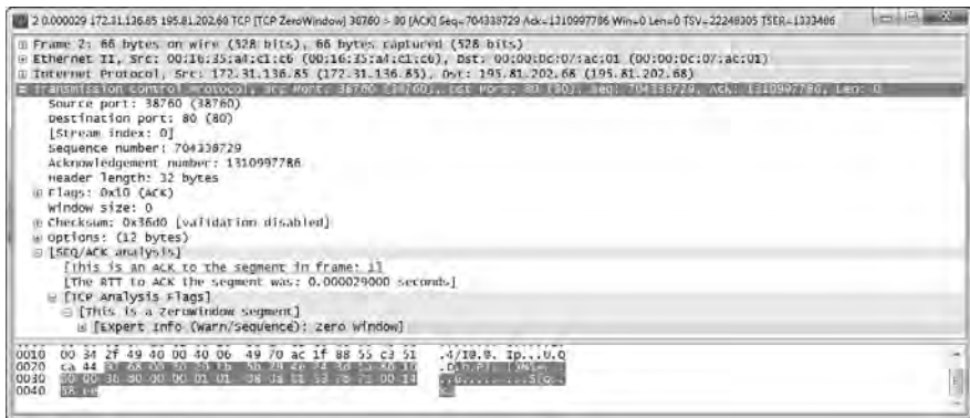
Figure 9-19: Zero window packet halting data transfer
