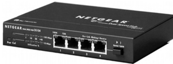
Figure 1-4: A typical 4-port Ethernet hub
