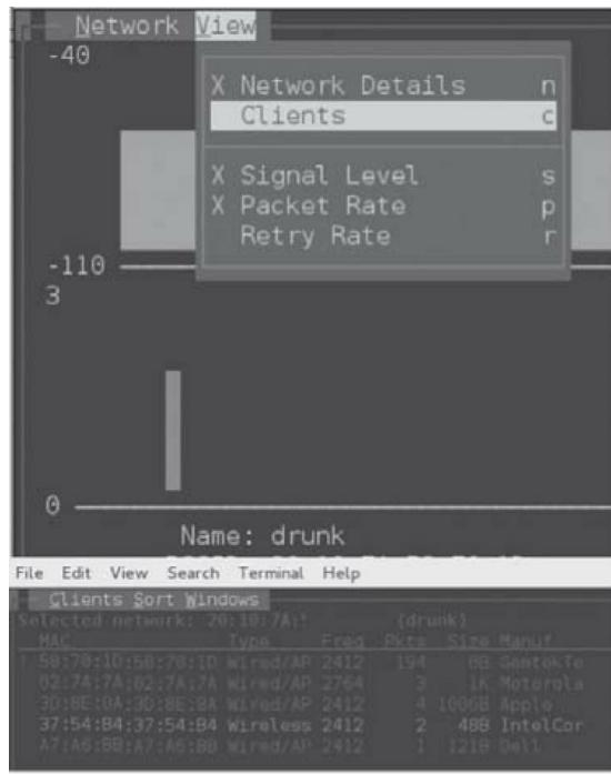
Figure 117 - Finding Clients Connected to an AP
