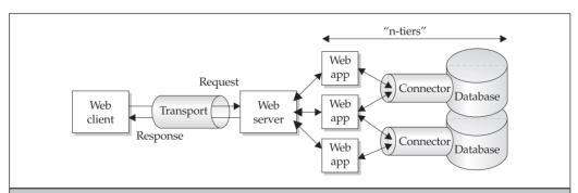
Figure 1-1. The end-to-end components of a typical Web application architecture
