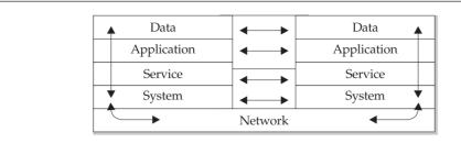
Figure 1-2. A layered model for network, system, service, application, and data-related vulnerabilities
