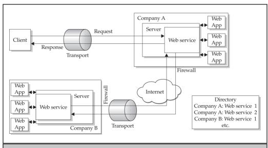
**Figure 10-1.** A diagram of a stereotypical Web services architecture
