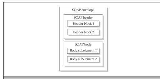
**Figure 10-2.** A schematic representation of a SOAP message, showing envelope, body, and headers
