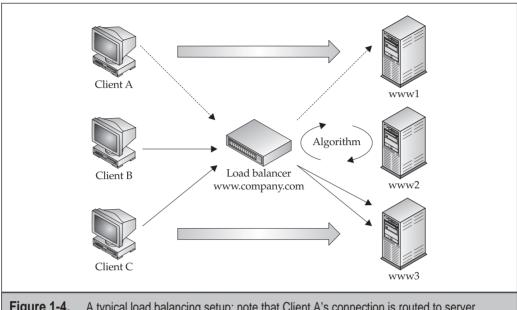
**Figure 1-4.** A typical load balancing setup; note that Client A's connection is routed to server www1, while Clients B and C are routed to server www3 based on the load balancer's algorithm
