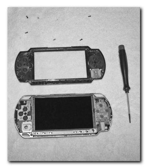
FIGURE 4-6: The first layer of PSP guts
