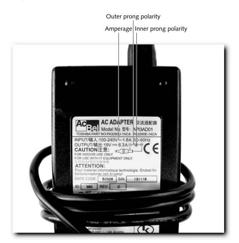
FIGURE B-1: Determining the polarity of a power supply
