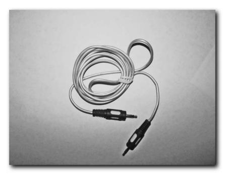
FIGURE 11-2: Dual-male 3.5 plug stereo audio cable
