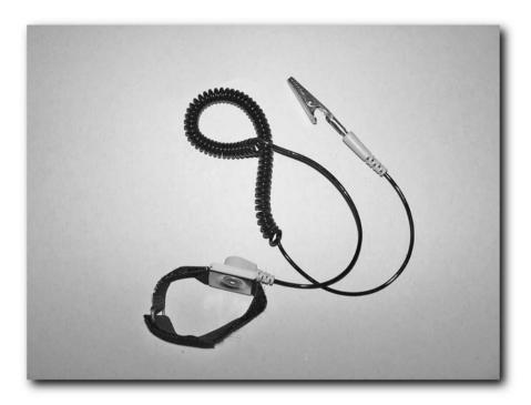
FIGURE 4-3: The electrostatic wrist strap
