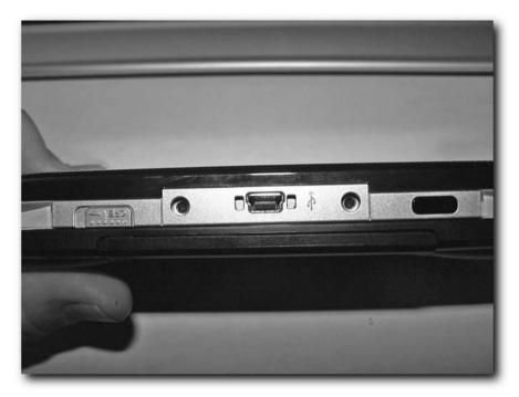
FIGURE 3-13: The USB port on the PSP
