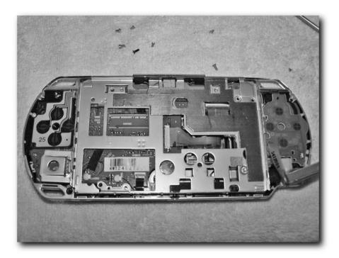
FIGURE 4-11: The metal screen holder with the nine screws removed
