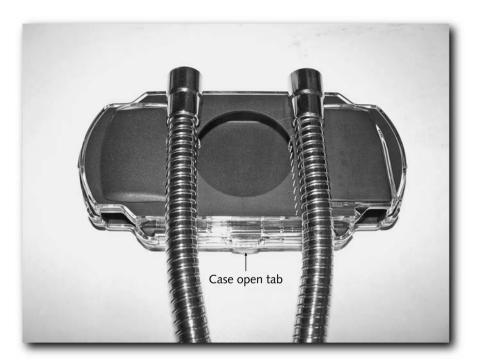
FIGURE 14-17: Make sure the case opening tab is facing you
