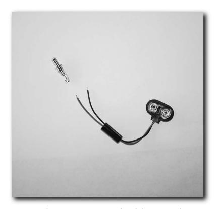
FIGURE 13-10: The snap connector wires run through the DC power plug's casing
