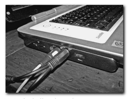
FIGURE 11-4: The audio cable properly connected
