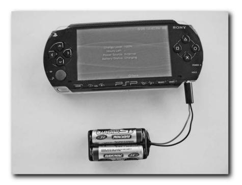
FIGURE 13-12: The external battery pack in action
