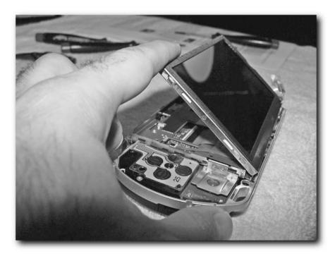
FIGURE 4-9: The screen partially removed
