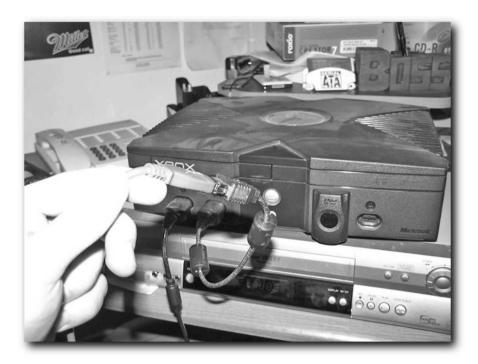
FIGURE 3-17: Connecting the Xbox adapter
