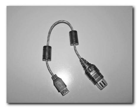
FIGURE 3-15: The Xbox Controller USB Adapter
