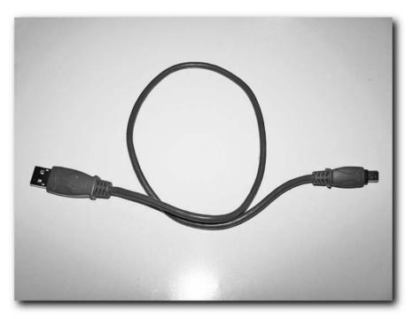
FIGURE 3-12: A mini-USB to full-size USB cable
