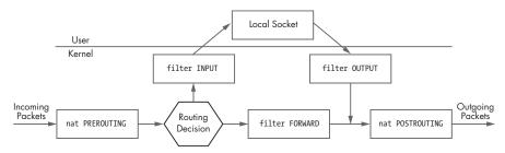
Figure 1-1: iptables packet flow
