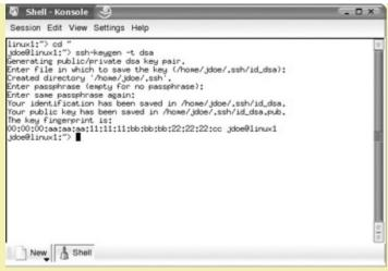
Figure 10-4: Generating SSH keys
