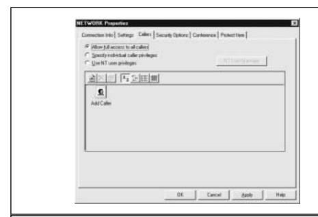
Figure 13-2. pcAnywhere 8.0's default authentication is set to Allow Full Access To All Callers
