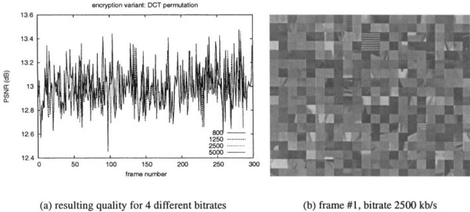
Figure 5.3. DCT block permutation, results with test sequence #4
