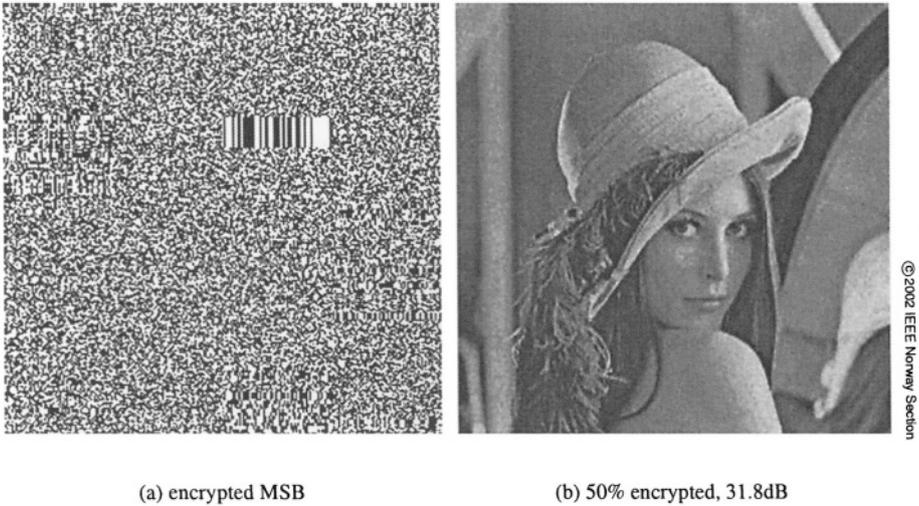
Figure 5.48. Further visual examples for selective bitplane encryption.
