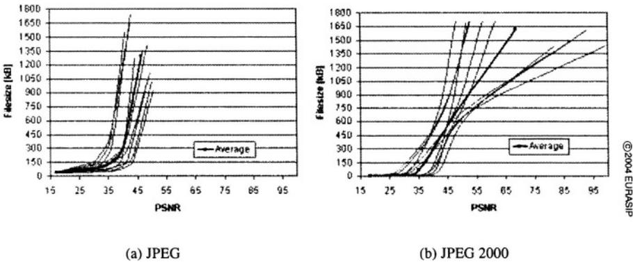
Figure 4.3. Rate-distortion performance of JPEG and JPEG 2000.
