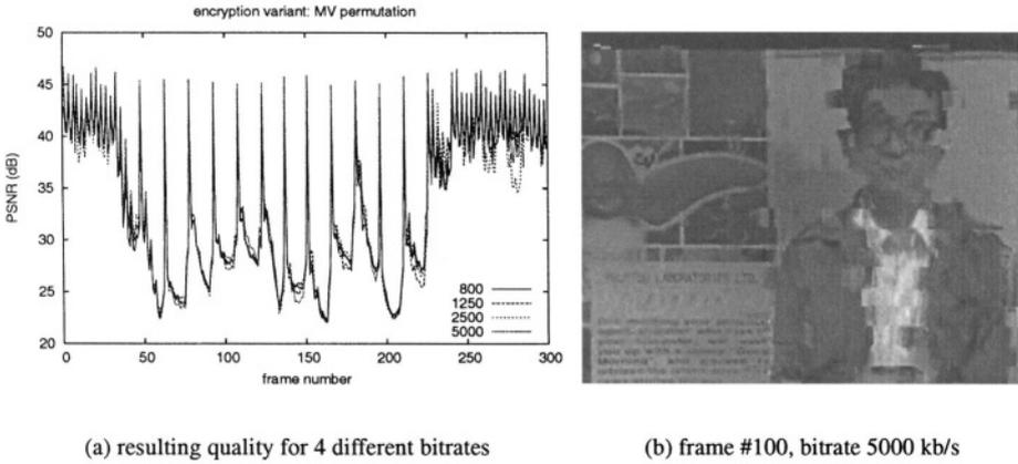
Figure 5.4. Motion vector permutation, results with test sequence #1
