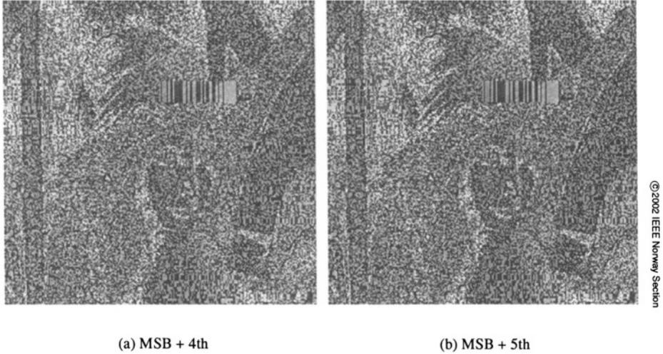
Figure 5.49. Visual examples for encryption of MSB and one additional bitplane.
