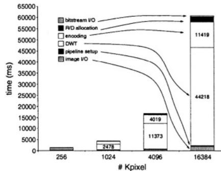
Figure 4.1. Runtime analysis of JJ2000 compression for increasing image size
