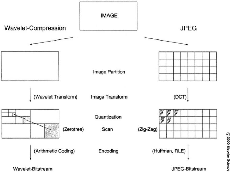
Figure 2.4. Comparison of DCT-based and wavelet-based compression schemes
