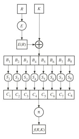
The operation is illustrated above. We may note that E and  $\pi$  are linear operations, in other words, they could be replaced by multiplication of a bit vector by a matrix. On the other hand,
