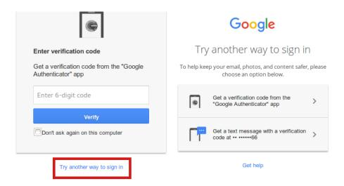
Fig. 4: Bypassing dedicated 2FA apps. The screenshot on the left shows Google 2SV requesting a verification code from the Google Authenticator. Note the *Try another way to sign in* option near the bottom of the window. When clicked, the right-hand figure shows the fallback option to get a text message with an OTP sent over SMS. An attacker in control of the PC-browser is therefore able to dicate what 2FA technique is used.
