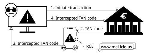
Fig. 2: Completing fraudulent transactions while bypassing 2FA. After our app processes the TAN code, it loads a remote webpage into a **WebView** component that allows the attacker to perform Remote Code Execution (RCE). This way, attackers can hide their malicious activity from Google Play.
