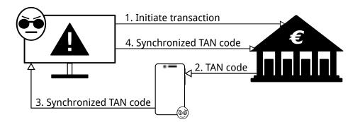
Fig. 3: Breaking 2FA on Apple Continuity. If enabled, Mac OS X 10.10 automatically synchronizes SMS messages between different Apple devices, breaking the second factor.
