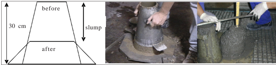
Figure 2. Testing process using the Abrams cone
