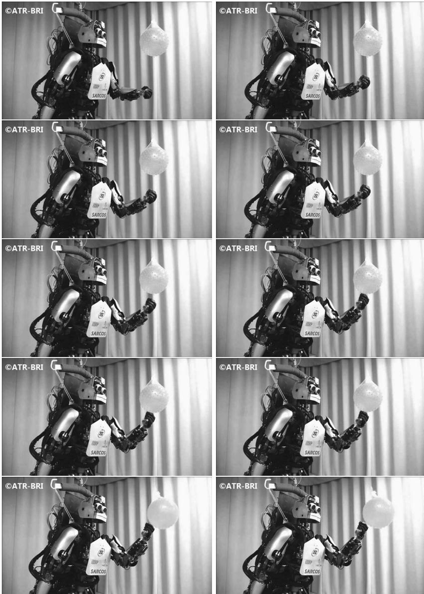
**FIGURE 9.13:** Typical example of arm reaching using the policy obtained by the IW-PGPE-OB method (from left to right and top to bottom).
