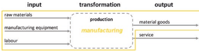
Fig. 2.1 Manufacturing as a transformation process to create material goods as an output
