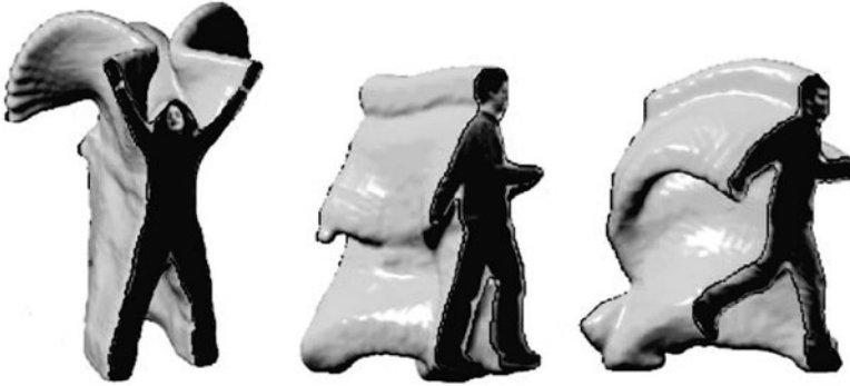
Fig. 9.3 Example space–time volumes spanned by actions of jumping, walking, and running. Figure courtesy [18]
