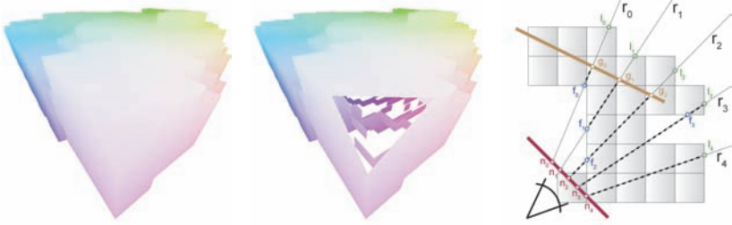
Figure 11.5. When the near clipping plane intersects the volume, some rays must be started at the near clipping plane (left) in order to avoid wrong ray starting positions (center). Near clipping and termination of rays at scene geometry intersections must be combined correctly (right). The volume is shown subdivided into small bricks for efficient empty-space skipping. (Images reprinted from [232]. © Eurographics Association 2006.
