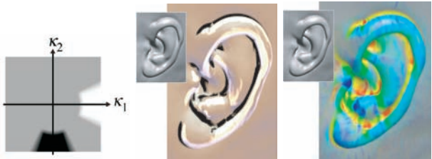
Figure 14.17. Visualizing specific shapes such as ridge and valley lines by simply painting them in the 2D curvature domain. (Images courtesy of Gordon Kindlmann, © 2003 IEEE.)
