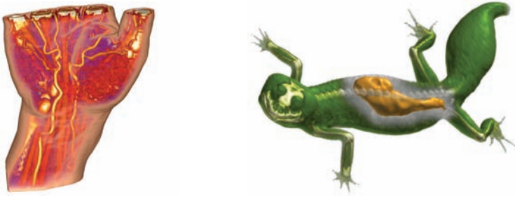
Figure 15.15. View-dependent transparency in volume illustrations. The left image demonstrates context-preserving volume rendering. The right image shows an example of importance-driven volume rendering that allows us to view the inner parts of the gecko. Left image courtesy of S. Bruckner, S. Grimm, A. Kanitsar, and M. E. Gröller [19], © Eurographics Association, 2005. Right image courtesy of I. Viola, A. Kanitsar, and M. E. Gröller [272], © 2004 IEEE.
