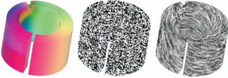
Figure 14.26. Image-space flow advection on curved surfaces. The vector field (left) is projected to image space and advects noise patterns (center) in the projected directions, which results in the illusion of flow advection on the surface in 3D (right). (Images courtesy of Bob Laramée [153], © 2003 IEEE.)
