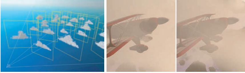
Figure 11.1. A powerful combination of volume and billboard rendering is to use billboards as impostors [2], e.g., for cloud rendering (left). The cached impostor images are updated only when the error with respect to the real view becomes too large [94, 233, 237]. A major problem of using billboards or impostors are potential clipping artifacts where they intersect scene geometry (center). (Images courtesy of Mark Harris [97].)
