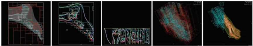
Figure 17.14. Gradient subtextures defined by the boxes enclose all the voxels of similar densities and nonzero gradient magnitude (left two images). The gradient subtextures are packed into a single texture (middle). Resulting rendering of the foot with mixed boxes and textures (right two images). (Images courtesy of Wei Li and Arie Kaufman [162], © 2003 Canadian Information Processing Society.)
