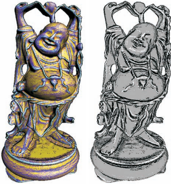
Figure 14.23. Happy buddhas. The left image uses the 1D curvature transfer function depicted in Figure 14.22 to visualize maximum principal curvature. The right image uses the 2D curvature transfer function depicted in Figure 14.17 to highlight ridge and valley lines in white and black, respectively. Note that no actual lines are drawn. These images were generated using ray casting on a 256 \times 256 \times 512 distance-field volume [93]. No geometry was used.
