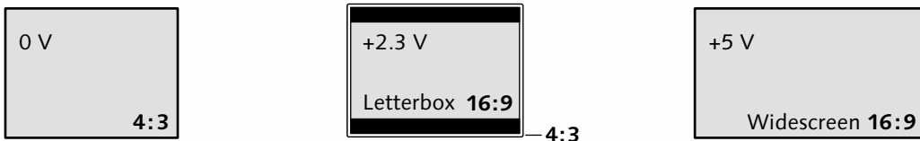
Figure 34.11 S-video widescreen signalling
