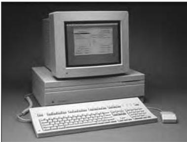
The Mac IIx used the same “Open Mac” case as the original Mac II, but came standard with dual 1.44MB 3.5-inch disk drives and was easier to upgrade.
