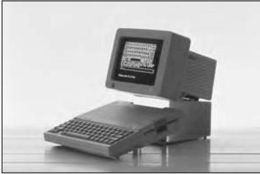
The Apple IIc, shown here with an optional monochrome monitor, packed all the power of the Apple IIe into a very compact case.
