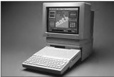
The Apple IIc Plus, shown here with an optional color monitor, had many different code names and featured a built-in 3.5" disk drive, more memory, and a much faster CPU.
