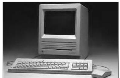
The Mac SE was the first model with an optional internal hard drive and PDS (processor direct slot); hence the name, which stands for “system expansion.”
