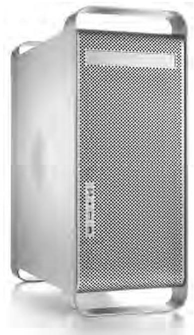
Equipped with dual 2GHz 64-bit PowerPC G5 processors, at its introduction the Power Mac G5 was the world’s fastest PC.
