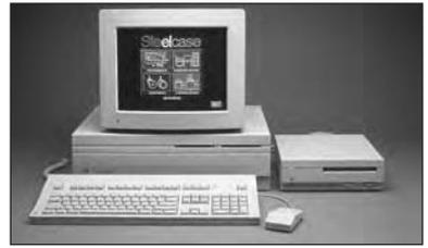
The Mac II (shown here with an optional external SCSI CD-ROM drive) was the first Macintosh designed to be easily opened and expanded by end users.
