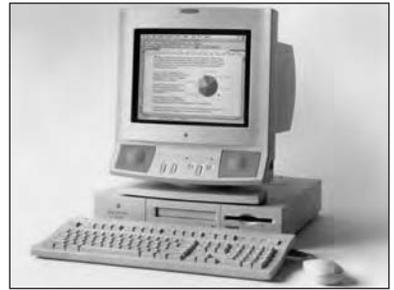
Apple's first new Macs of 1995 (such as the Power Mac 6100 shown here) were marginally faster versions of the Power Macs introduced less than a year before.
