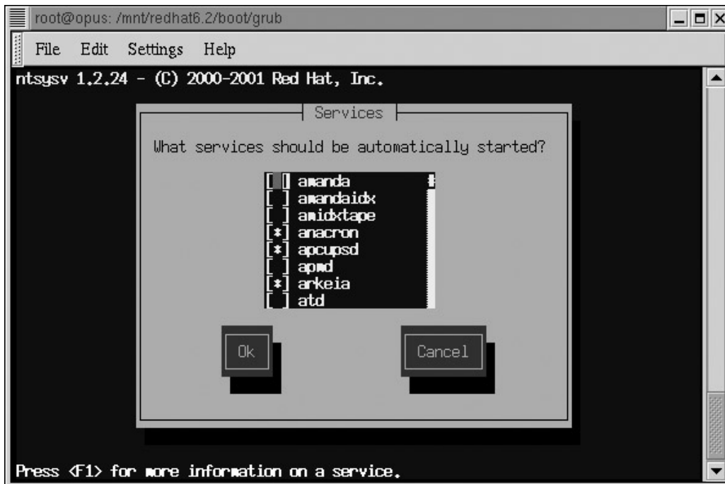
Figure 3.2: Use the ntsysv utility to control which services are automatically started at bootup. Another tool for adding, deleting, or reordering services in run levels 2–5 is the tksysv utility, which is available as part of the Red Hat distribution. This utility is X-based and is quite good. It presents a display of each of the services that are started and stopped at the various run levels and allows you to delete or add as needed. The principles of its use are basically the same as for ntsysv. Figure 3.3 shows the tksysv utility.
