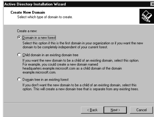
Figure 4.7 The Create New Domain Dialog Box Used for Creating a New Domain in a New Forest
