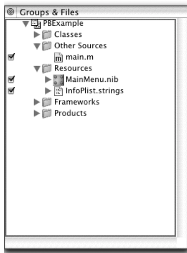
Figure 3.10 The Contents pane provides access to project file, libraries, and resources such as images.
