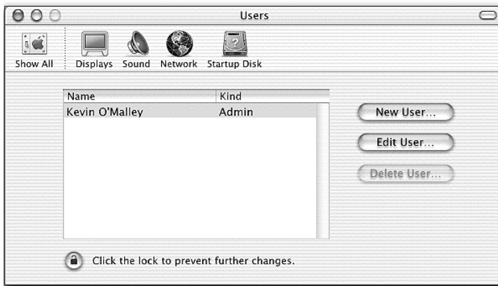
Figure 2.5 You add users to the system and assign administrator privileges using the System Preference program’s Users pane.
