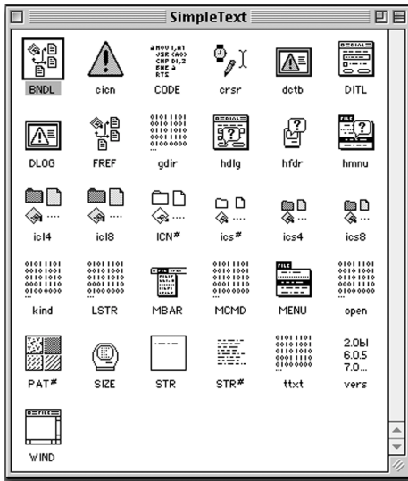
Figure C.4 An application's resource fork, like the SimpleText editor, is composed of many resources that collectively form an application.
