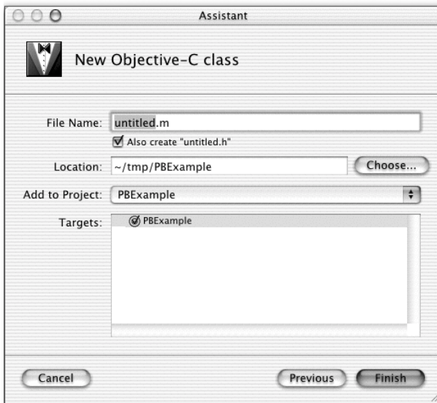
Figure 3.20 When creating a new class file, Project Builder displays the New Objective-C class window. Use this window to specify the name of the class and its location.
