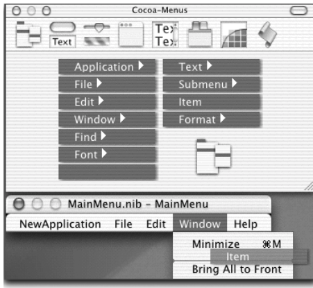
Figure 3.26 You use the Cocoa Menus item to create and edit your application's menu.
