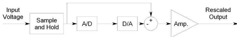
Fig. 15.1. A single unit of a pipelined A/D
