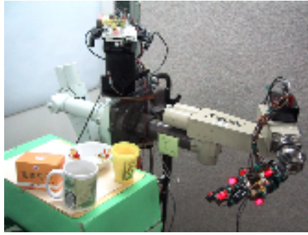
Fig. 7.10. Arrangement of objects for Experiment 2. Metalman is required to grasp one of the cups (selected interactively) and pour the contents into the bowl.
