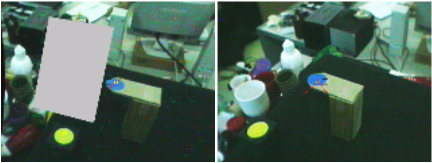
(a) Initial pose of object and virtual obstacle (shown in grey). The gripper is outside the field of view and initially tracked using only kinematic measurements.
