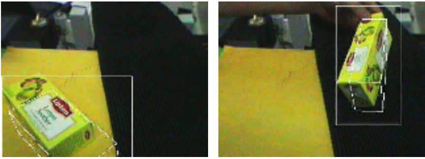
(a) Frame 150: failure for edge only tracker due to low contrast background
