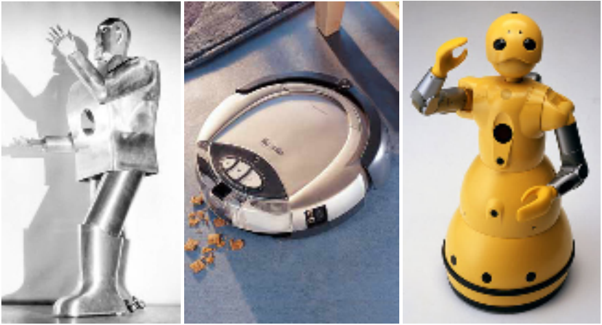
Fig. 1.1. Service robots of the past, present and future. Elektro (left) was built by Westinghouse in 1937 and exhibited as the ultimate appliance, although it was little more than a complex automaton. Present-day service robots such as the Roomba (centre) from iRobot can perform specific tasks such as vacuum cleaning autonomously, but have limited application. The concept robot Wakamaru (right) from Mitsubishi is designed to develop its own motivations to help in the daily life of its user, and represents the first generation of universal aids. Elektro image from http://davidszondy.com/future/robot/elektro1.htm . Roomba image from http://www.frc.ri.cmu.edu/hpm/talks/Extras/roomba.JPG . Wakamaru image from http://www.expo2005.or.jp/jp/C0/C3/C3.7/C3.7.5/ .
