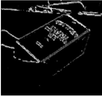
(a) Edge filter output (grey-level indicates edge orientation)
