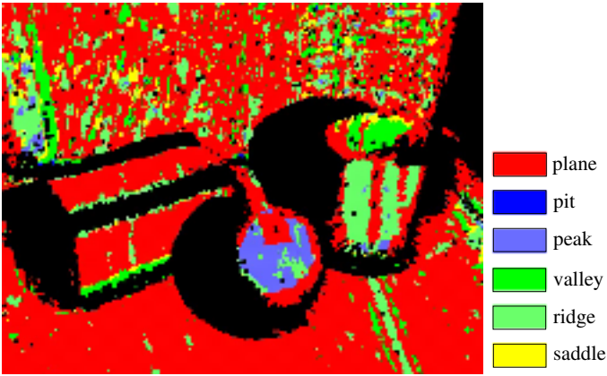
Fig. 4.14. Curvature-based surface type result (compare to Figure 4.10(b)).
