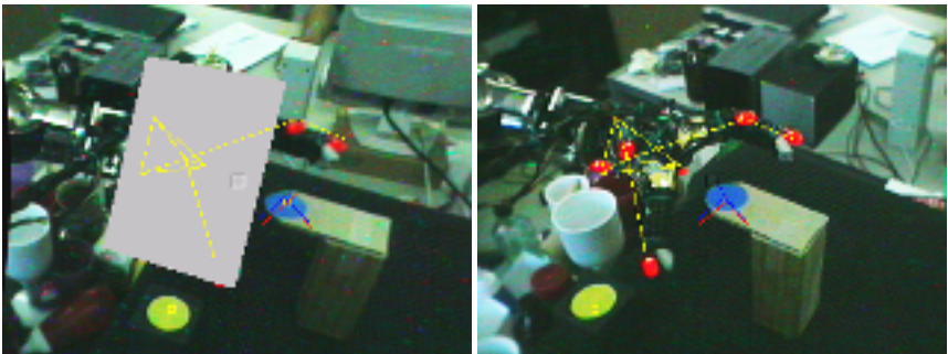
(c) Final pose at completion of the servoing task. The gripper is obscured by the virtual obstacle in the left visual field, leaving only monocular feedback.
