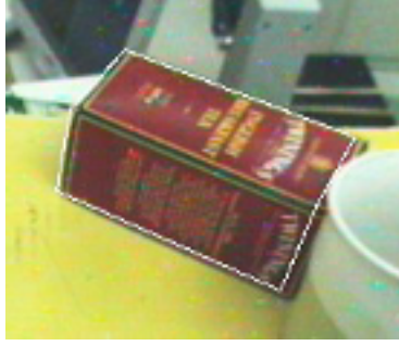
(a) ROI in initial image with outline showing pixels used for creation of object colour filter
