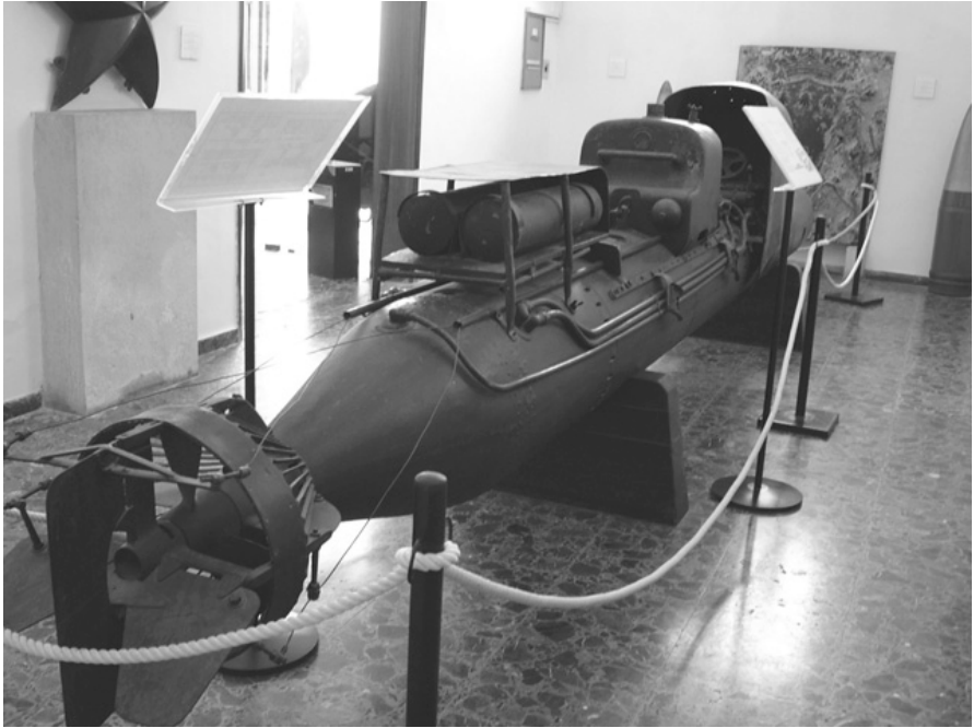
Fig. 1.5. Pig , manned vehicle used by the Royal Italian Navy during the second world war in the Mediterranean Sea. The thruster and the group rudder/stern can be observed in the bottom left angle of the photo
