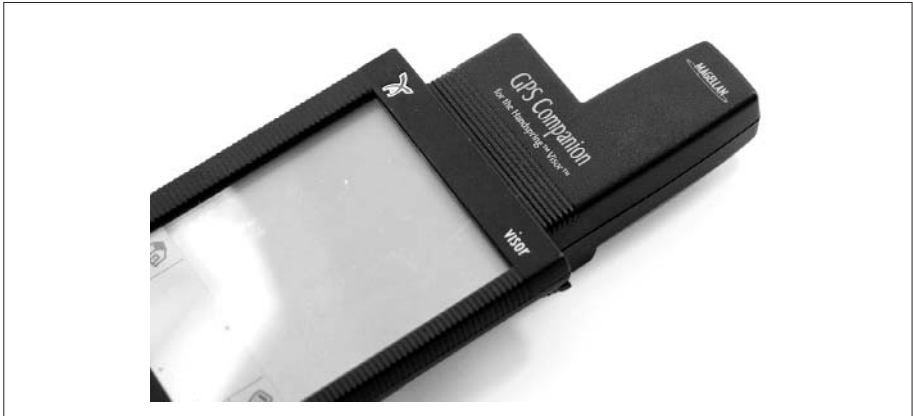
Figure I-8 The Handspring Visor looks much like a Palm III, but features the Springboard expansion slot in back.
