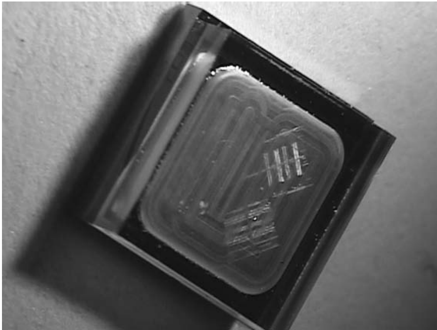
FIGURE 4.23 A surface micromachine encapsulated by a piece of glass. Comb-drives can be seen through the right side of the mechanically machined cap. This process can be accomplished either on a die or wafer basis. (Photograph courtesy of A. Oliver, Sandia National Laboratories).
