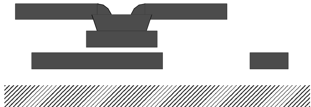
FIGURE 4.35 A cross section of the pin and socket joint where the pin has moved out of the joint.
