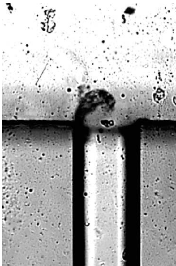
FIGURE 9.2 Experimental snapshot of the microchannel junction. The silica channel and the latex colloids are oppositely charged, and hence both electrophoretic and electroosmotic motions are in same direction. The picture shows a spiral colloidal aggregation at the inner corner.
