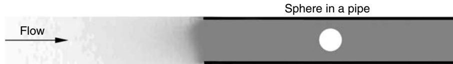
FIGURE 6.10 Velocity contours for a sphere in a pipe in the transitional flow regime ( Kn = 3.5 ). Molecules reflected from the sphere create a diffusive layer at the entrance of the pipe [Liu et al., 1998].
