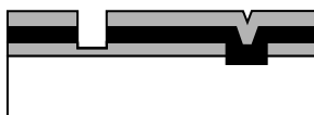
FIGURE 16.93 Masking and process sequence preparing a wafer for laterally grown porous polysilicon. (From Field, L., Low-Stress Nitrides for Use in Electronic Devices (University of California, Berkeley, 1987), pp. 42 and 43. With permission.)
