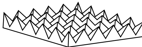
FIGURE 31.8 Chemically etched orthogonal, triangular groove wick. (From Mallik, A.K., and Peterson, G.P. (1991) in 3rd ASME–JSME Thermal Engineering Joint Conf. Proc. , Vol. 2, March 17–22, Reno, NV, pp. 394–401. With permission.)
