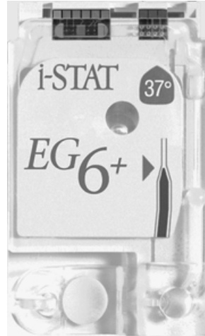
FIGURE 6.2 Blood sample cartridge using microfluidic channels. (Courtesy of i-Stat, East Windsor, NJ.)
