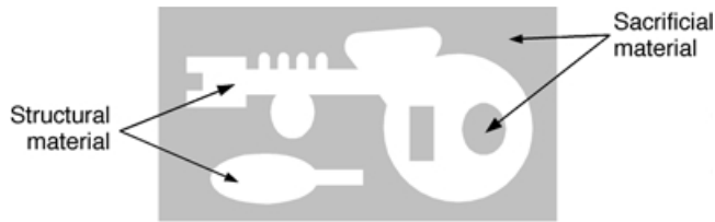
FIGURE 19.9 Plane view of a typical layer in EFAB, depicting structural material and surrounding sacrificial material.
