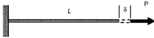
FIGURE 27.4 Illustration showing the elongation of a column. L is the original length of the column, and \delta is the change in the length of the column.
