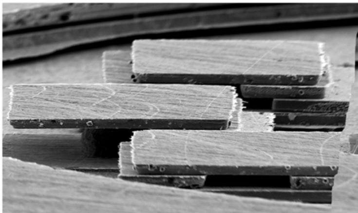
FIGURE 19.16 Some five-layer nickel structures measuring \sim 40 \mu\text{m} high.
