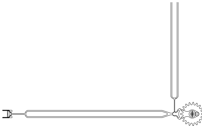
FIGURE 27.16 Detail of Figure 27.15 showing the thin linkages that connect the comb drives to the gear.
