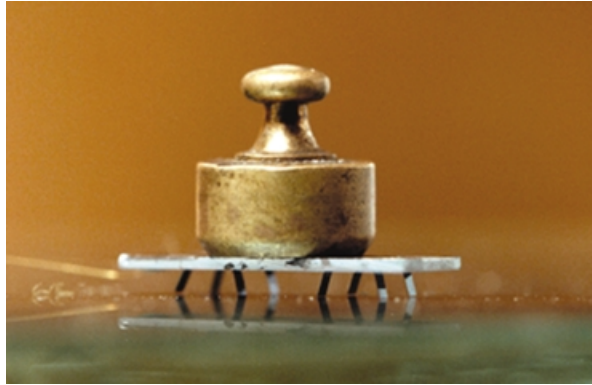
COLOR FIGURE 28.17 Photograph of the microrobot platform used for walking during a load test. The load of 2500 mg is equivalent to maximum 625 mg/leg (or more than 30 times the weight of the robot itself). The power supply is maintained through three 30- \mu\text{m} -thin and 5- to 10-cm-long bonding wires of gold. The robot walks using the asynchronous ciliary motion principle described in Figure 28.6c. The legs are actuated using the polyimide V-groove joint technology which was described in Figure 28.10. (Photo by P. Westergård; published with permission.) (Note: Videos on different experiments that have been performed using the microrobot shown above are available at: http://www.s3.kth.se/mst/research/gallery/microrobot_video.html .)
