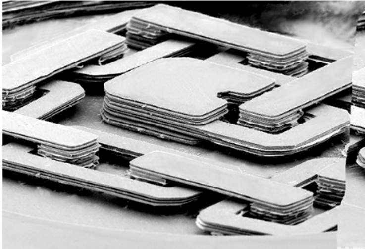
FIGURE 19.17 A 12-layer microchain fabricated in nickel using EFAB, without assembly. Overall height is \sim 100\ \mu\text{m} and the width of a chain link is \sim 290\ \mu\text{m} . All horizontal links are free to move.
