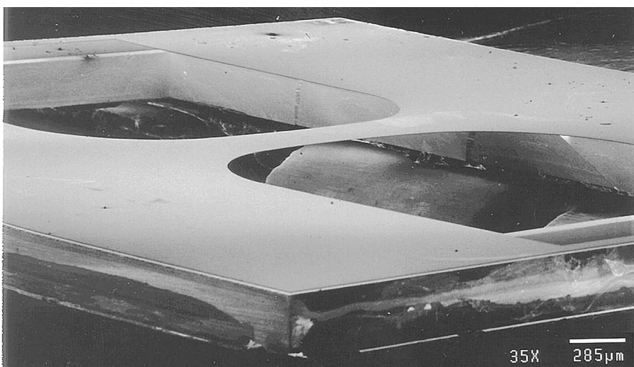
FIGURE 3.2 Scanning electron micrograph of a polysilicon tensile specimen in a supporting single-crystal silicon frame. (From Sharpe, W.N., Jr., Yuan, B., Vaidyanathan, R., and Edwards, R.L. (1996) Proc. SPIE 2880 , pp. 78–91. With permission.)
