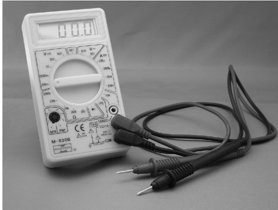
PHOTO 2.5 A multimeter – the one used throughout this book – although any multimeter with at least the specification given will do.
