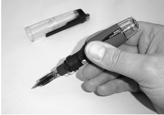
PHOTO 12.13 A gas-powered soldering iron. Butane gas is used to power the iron, and a single charge can give 20 minutes or so of use. These soldering irons are very useful where mains power is unavailable.
