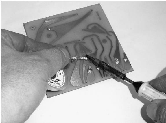
PHOTO 12.39 Desoldering using solder braid – the molten solder wicks into the strands of the solder braid away from the joint.
