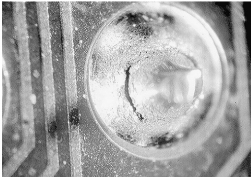
PHOTO 12.9 Cracked joints – the joint has probably been moved before it was cool, causing the solder to crack. This particular joint may work at the moment, but will probably fracture totally soon (ECS).
