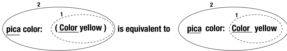
Figure 11-2. Unary message sends are executed first, so Color yellow is executed first. This execution returns a color object, which is passed as the argument of the message color: ... that is sent to pica .
