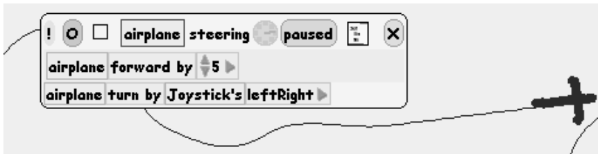
Figure 24-17. Now the joystick's leftRight variable will control the turning of the airplane.
