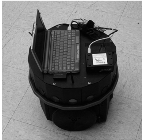
Fig. 1. Bob: a test platform for the PRISM Mobile Robot software.
