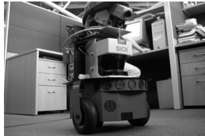
(d) A Pioneer indoor robot equipped with a camera and a SICK laser
