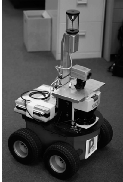
(b) A Pioneer2AT equipped with two cameras and a SICK laser
