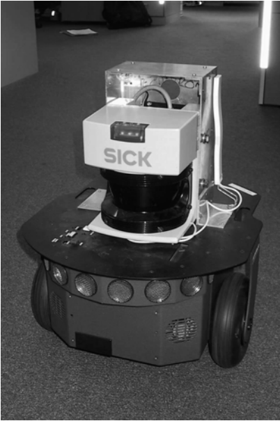
(a) A Pioneer indoor robot equipped with a SICK laser
