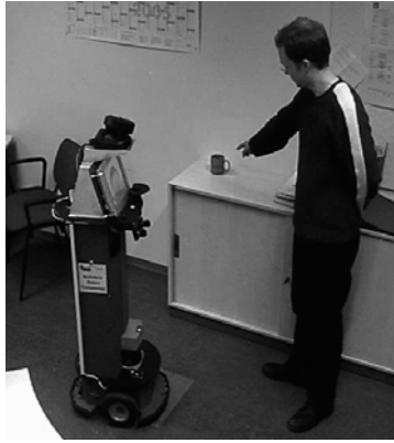
Fig. 7. A user teaching an object to the mobile robot BIRON.
