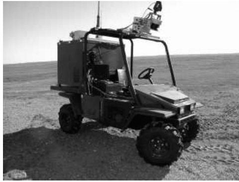
Fig. 10. One of two modified Koyker Raptors used in DRDC's ALS Project. Each Raptor used one or more roof mounted SICK lasers and stereo cameras; Differential GPS and IMU; and wireless mesh networking routers.
