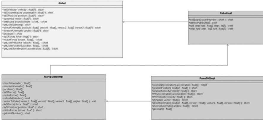
Fig. 3. Particular of Penelope class Diagram with RobotImpl inheritance structure and Puma200Impl interface (attributes and methods).
