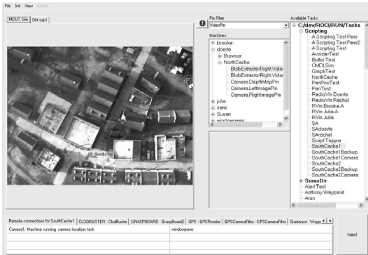
Fig. 2. ROCI Browser during the execution of a multi-robot mission: It is possible to monitor the status of each node, the tasks and modules being executed and even see the real time location of each robot on a map.
