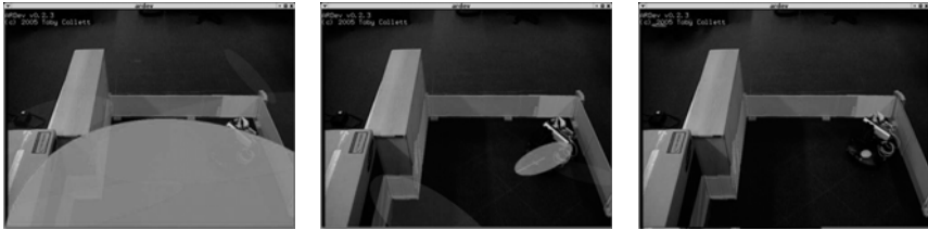
(g) AMCL Initial Distribution, High Covariance (h) AMCL Improved Estimate (i) AMCL Converged Result
