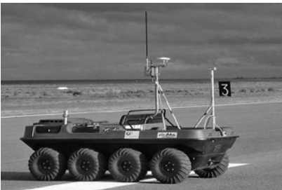
(e) An Argo unmanned all-terrain ground vehicle
