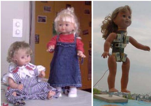
*Figure 20.1.* Left Picture: On the left, the first prototype of Robota doll made out of LEGO, and, on the right, the second prototype of Robota doll. Right Picture: The new commercial prototype (version Caucasian).
