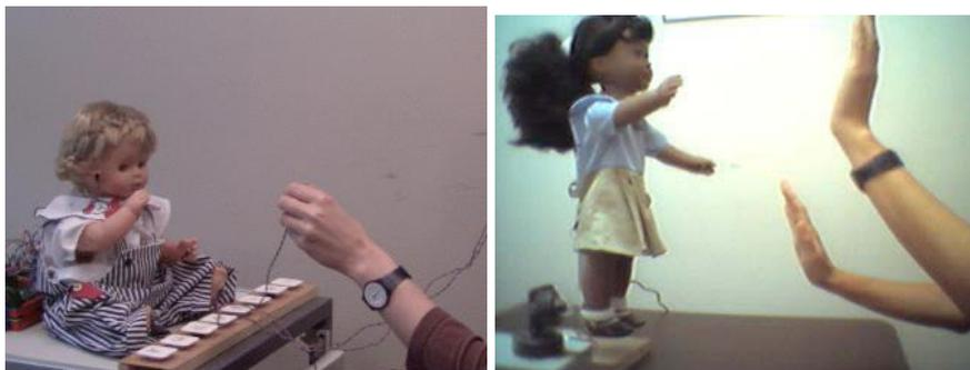
*Figure 20.2.* Left: The teacher guides the motions of Robota using a pair of glasses holding a pair of IR emitter. The glasses radiate which can be picked up by the robot's "earrings" IR receptors. Right: Robotina, the latino version of Robota mirrors the movements of an instructor by tracking the optical flow created by the two arms moving in front of the camera located on the left side of the robot.
