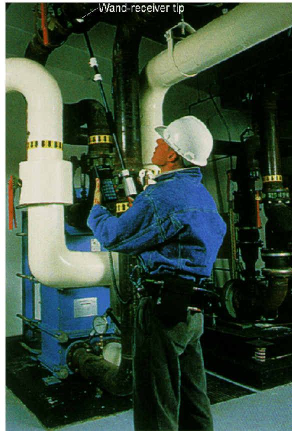
Figure 6.27: In its originally intended hand-held mode of operation the surveyor places the tip of the wand-receiver at a point of interest to record that point's 3-D coordinates. (Courtesy of Spatial Positioning Systems, Inc.)
