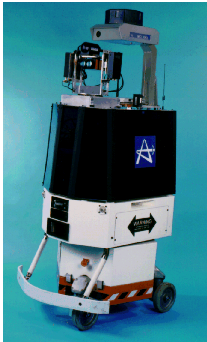
Figure 7.2: The ARK system is based on a modified Cybermotion K2A+. It is one of the few working navigation systems based on natural landmark detection. (Courtesy of Atomic Energy of Canada Ltd.)
