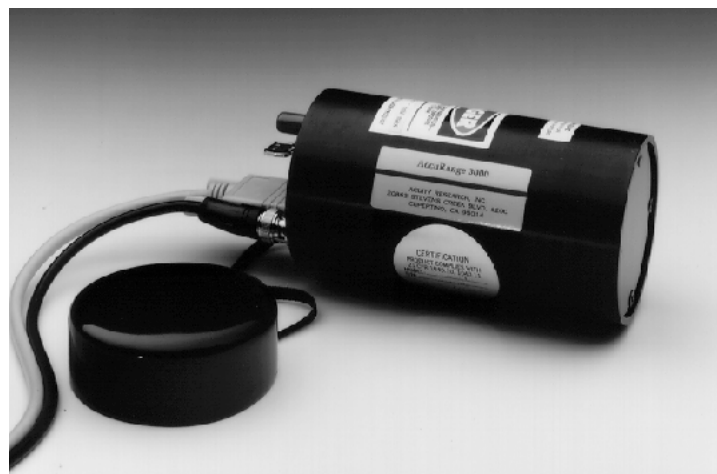
Figure 4.26: The AccuRange 3000 distance measuring sensor provides a square-wave output that varies inversely in frequency as a function of range. (Courtesy of Acuity Research, Inc.)
