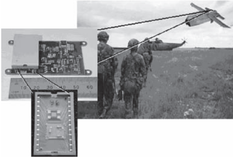
Figure 21.3.6: The SnifferSTAR is a nano-enabled chemical sensor integrated into a micro unmanned aerial vehicle. (Courtesy of Sandia National Laboratories, Albuquerque NM, and Lockheed Martin Corp.)
