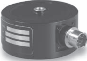
Figure 11.3.7: Typical general-purpose load cell.
