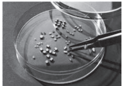
Figure 5.2.11: Multiple MEMS accelerometer flexure containing diffused and metallized piezoresistive gages in Wheatstone bridge configuration.
