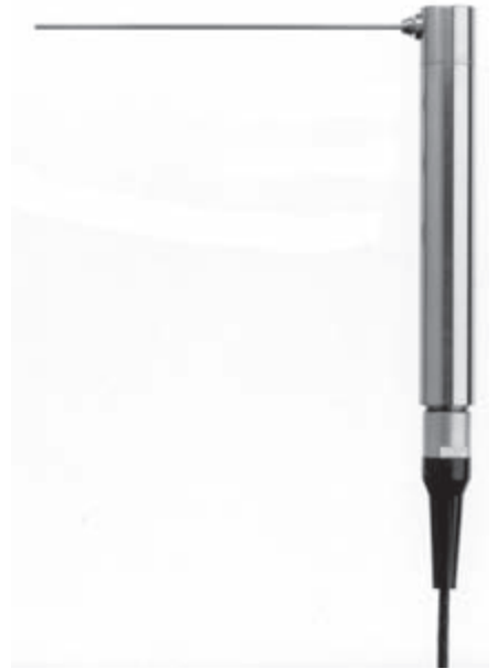
Figure 18.9.3: Probe microphone. (Courtesy of G.R.A.S. Sound and Vibration.)
