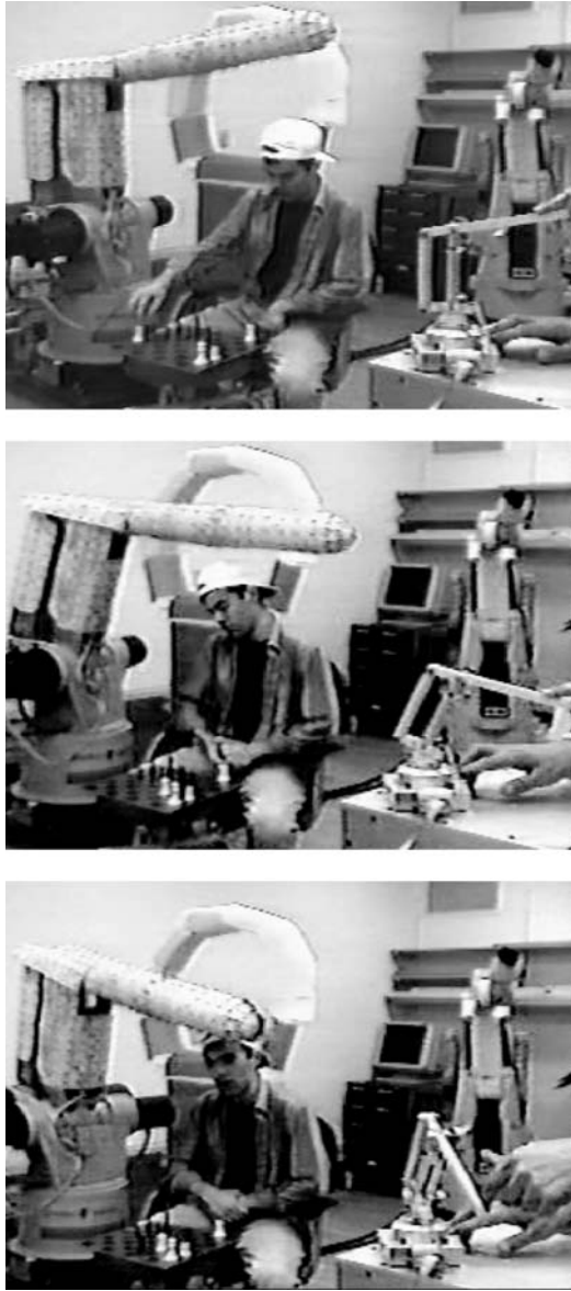
Figure 8.11 Robot teleoperation. Here the operator has attempted “to hurt” a student sitting in the robot work space. After bringing the (slave) robot right above the student’s head (second picture), the operator moves the master arm sharply down, “expecting” the robot to repeat this motion. Note the difference between the robot and master arms’ positions (second picture); the latter shows a clear intention to bring the robot much lower than it went. Eventually the operator moves the master arm toward us, and the robot follows (third picture). Note: The videos that supplied pictures for Figures 8.9 to 8.11 can be seen in full on the web, http://aaaproduct.gsfc.nasa.gov/Project/public_html-NASA/LaRue-Lumelsty.htm .
