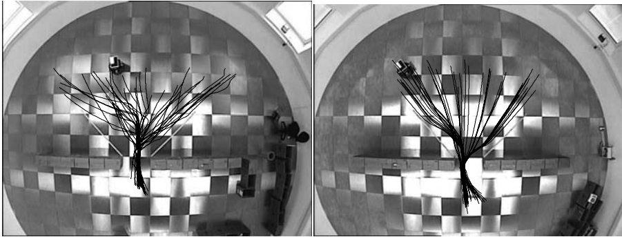
Figure 6.42. Left: The robot’s trajectories under manual control (39 runs, training data). Right: Trajectories taken under model control (41 runs, test data)
