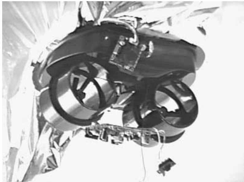
■ 14.7 A close-up of the turbo fan, miniature CCD camera, and TV transmitter
