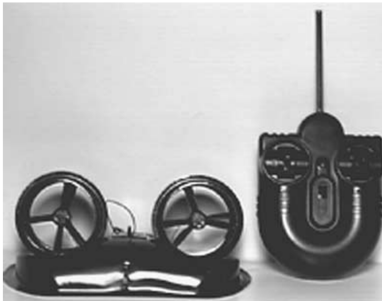
■ 14.5 Lightweight R/C control system for blimp
