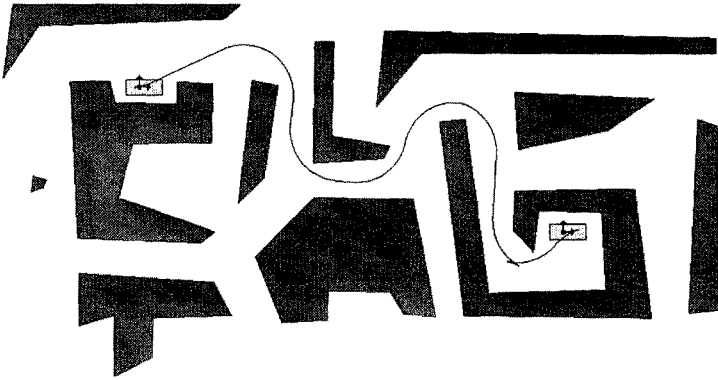
Fig. 12. A planned path for a car-like robot: the workspace is modeled by a grid of 250 \times 150 pixels; the total running of the algorithm is 2 seconds on an Indy Silicon Graphics.
