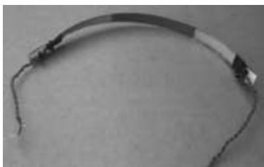
A bend sensor made from piezo film.
