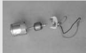
What the inside of a PM motor looks like.
