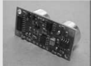
Ultrasonic sensors use the speed of sound to measure distance.
