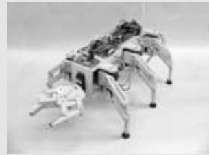
A walking robot can use linear motion to lift its legs for each step. Photo Jim Frye, Lynxmotion, Inc.
