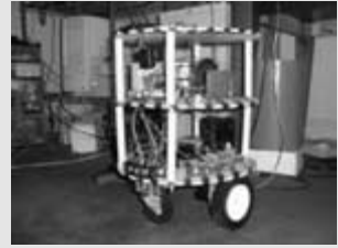
A teleoperated robot built by Michael Owings and operated by anyone with a Web browser.
