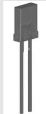
Phototransistors (and their cousins photoresistors and photodiodes) are used for simple robotic vision.
