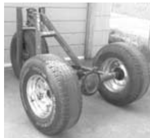
Beginnings of The Sentinel, with hacked-up General Motors differential. Courtesy Brad and Devon Graham.
