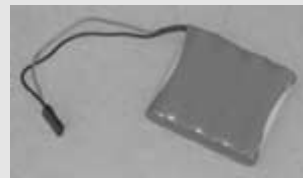
A typical battery pack for a consumer electronics device (in this case, a cordless phone).
