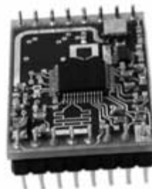
Model EWM-900-FDTC, 56-channel, full-duplex, 902-928 MHz data and audio transceiver module. Photo Radiotronic Inc.
