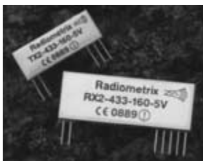
Model TX2/RX2 RF receiver and transmitter modules. Photo Radiometrix Ltd.
