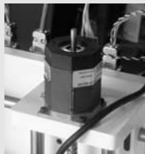
Stepper motors provide exact movement of the router for precision cuts.
