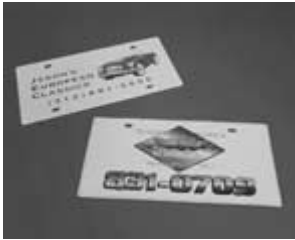
Making special license plates (adaptable to robotics) with heat transfer films. Photo Visual Communications.
