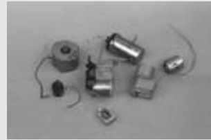
A variety of different motors types suitable for small robots.
