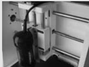
The router cuts and mills material by moving either the tool, the material, or both.
