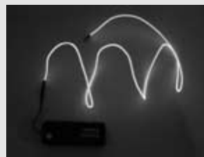
Electroluminescent is flexible "glow wire" that has both functional and decorative uses in robotics.
