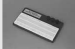
A typical electronics breadboard. They come in various sizes and styles.
