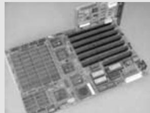
An old 486-class motherboard. One possible use for this relic is as a robot brain.
