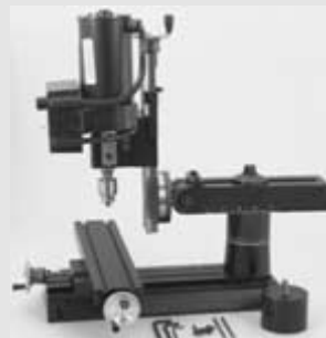
A desktop mill can be used to create miniature parts for your robot. Photo: Sherline Products Inc.
