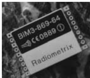
Model BiM3, 869/914MHz high speed FM radio transceiver module. Photo Radiometrix Ltd.
