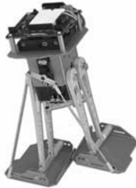
The Parallax Toddler walking robot. Photo Parallax, Inc.
