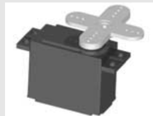
Model R/C servos are great for motorizing robots.
