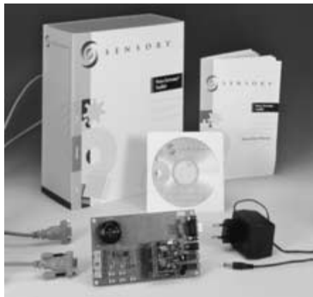
Voice Extreme Developer's kit, from Sensory. Photo Mario Galizia, Grafiche Galizia; Sensory, Inc.
