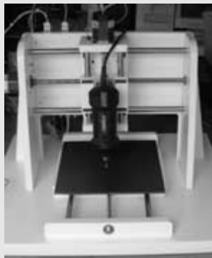
Gantry designs are typical of CNC routers.
