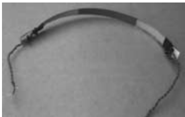
A bend sensor made from piezo film.
