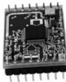
Model EWM-900-FDTC, 56-channel, full-duplex, 902-928 MHz data and audio transceiver module. Photo Radiotronix Inc.
