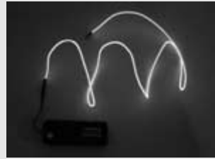
Electroluminescent is flexible "glow wire" that has both functional and decorative uses in robotics.
