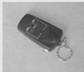
A key-ring transmitter from a store-bought wireless appliance control module.
