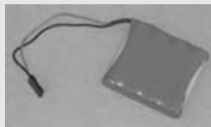
A typical battery pack for a consumer electronics device (in this case, a cordless phone).
