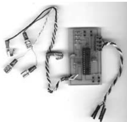
Model RCIC-2; a dual channel radio control interface with mixing. Photo Diverse Electronics Services.
