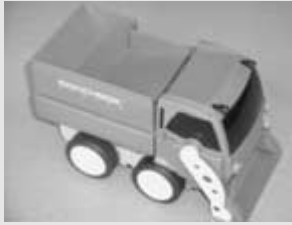
This Rokenbok radio-control "robotic" toy is outfitted with a linear motion forklift gripper.
