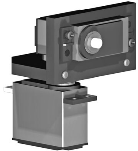
Figure 27-23 Complete X-Y joint, with servos.
