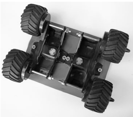
Figure 16-5 This 4WD robot base was constructed from two motorized toy models. The models used a single motor to power four wheels. For each motor the wheels on opposite sides were removed; a metal collar (fastened in place with a set screw) prevents the axle from coming out.
