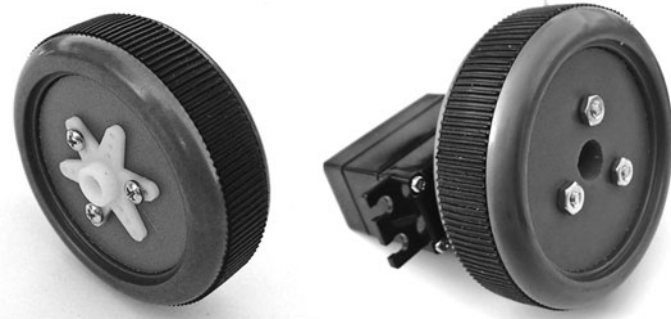
Figure 24-9 Most any kind of wheel can be converted for use with an R/C servo by attaching a servo horn to the side of the wheel. If your servo didn't come with an assortment of horns, you can purchase them separately.
