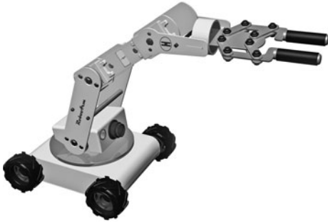
Figure 28-1 Robotic arm with three joints that each provide a degree of freedom.
