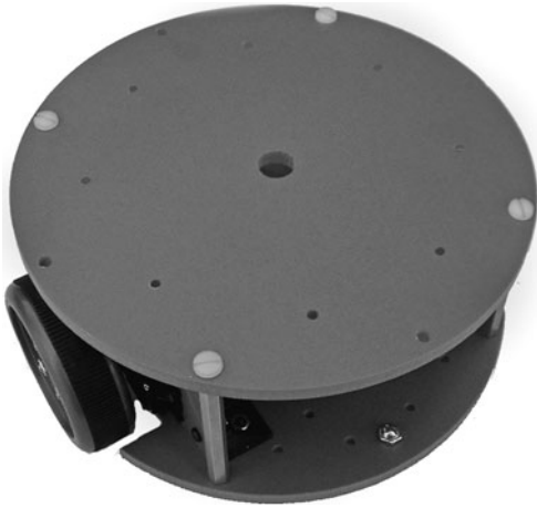
Figure 2-5 Small turtle-sized robots represent a class that's easy and inexpensive to build. They are ideal for learning about robotic design, construction, and programming.
