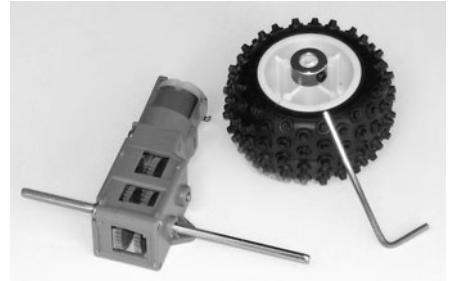
Figure 24-14 Metal collars may be used on wheels with an outsized hub (the hub protrudes from the wheel, giving more surface area to the shaft). Place the collar around the hub of the wheel. The compression tightens the hub around the motor shaft.
