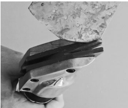
Figure 11-6 Air shears make quick work out of cutting sheet metal. Use a pencil to mark the line you want to cut, then slowly work the tool around the contours of the line.
