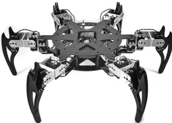
Figure 20-10 This six-legged hexapod robot uses 3 motors per leg, for a total of 18 motors. Because of the high number of motors, these kinds of robots are more difficult and more expensive to build. (Photo courtesy Lynxmotion.)
