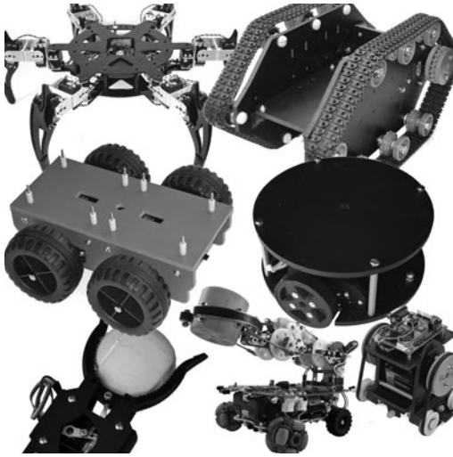
Figure 1-1 Amateur robots can take many forms and sizes: mobile (moving) robots use wheels, tracks, or legs for propulsion; arms and grippers allow the robot to manipulate its environment. (Includes photos courtesy Lynxmotion and Russell Cameron)
