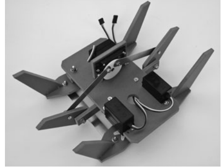
Figure 27-19 Under view of the completed Hex3Bot, showing how the middle legs are articulated using the servo.
