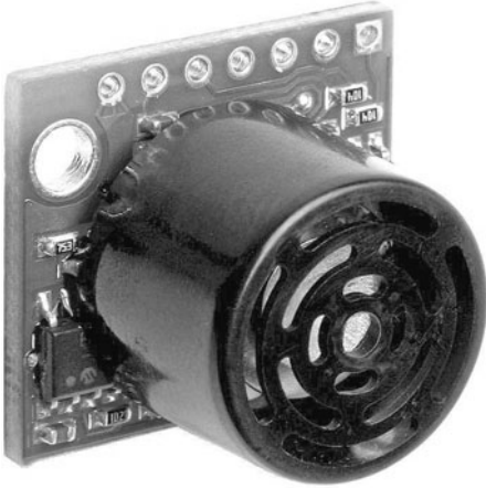
Figure 43-14 Ultrasonic distance sensor, using one transducer (both sends and receives sound). (Photo courtesy Maxbotics Inc.)
