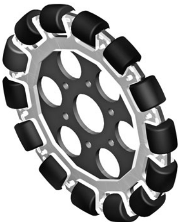
Figure 20-6 An example wheel used in a holonomic robot. Instead of a solid rubber tire, the rim of the wheel is composed of several rollers that are set at opposite angles to the rotation of the wheel.
