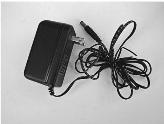
Figure 19-6 Wall transformer with a barrel plug. If purchasing a wall transformer for your robotics projects, make sure it provides the correct voltage and that the plug has the proper polarity to match your components.
