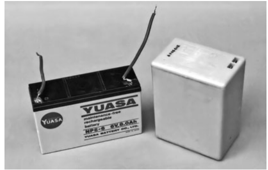
Figure 18-3 Sealed lead-acid (SLA) batteries are the largest and heaviest of the bunch, but they provide a lot of current, useful for larger robots.
