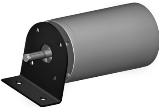
Figure 24-1 Motors with faceplate holes may use a flange for mounting. This method requires the proper size of machine screws; if the screws are too long, they'll interfere with the moving parts inside the motor.
