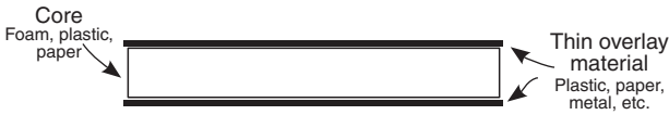
Figure 14-1 Substrates are constructed of sandwiching layers of materials together, each layer reinforcing the other. For very lightweight substrates, a foam core is layered top and bottom with a thick paper or plastic sheet.
