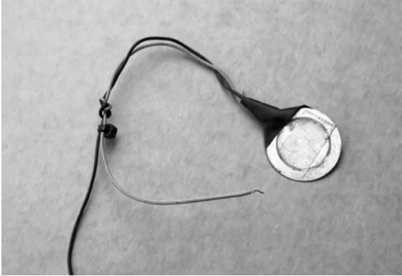
Figure 42-15 A homemade touch or “knock” sensor made with a piezoelectric disc, available as stand-alone components from many online electronics stores or in piezo speakers.
