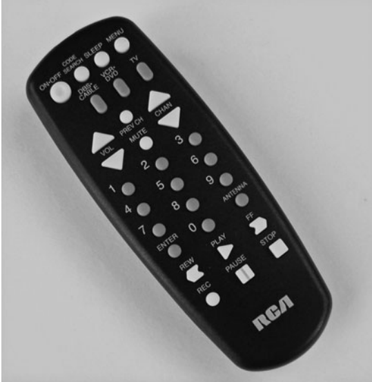
Figure 41-3 Example universal infrared remote control. To use a universal remote with the PICAXE microcontroller, you must select the code for a Sony TV, VCR, or other home electronics device.
