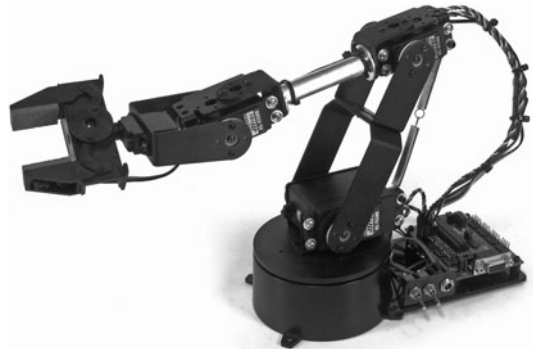
Figure 28-13 Robot arm kit, shown with control electronics and gripper. (Photo courtesy Lynxmotion.)
