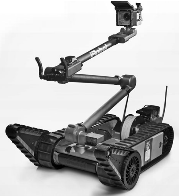
Figure 2-3 A telerobot requires a human operator to control it. The robot is usually semiautonomous, taking basic instructions via wireless feed and performing intelligent tasks. (Photo courtesy iRobot Corporation.)
