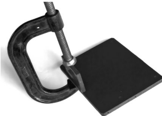
Figure 13-11 Clamping may be necessary to hold parts together while the adhesive sets and cures.
