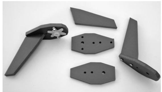
Figure 27-13 The front and rear legs, as cutout pieces and assembled. The rear legs have a six-arm "star" servo horn attached to them.
