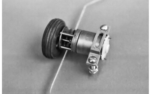
Figure 10-10 Ways to mount a motor using simple hardware and a flexible plastic strap. The technique works for motors with square or round cases.
