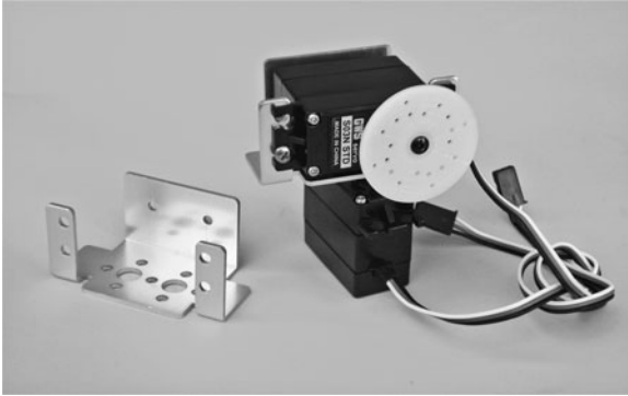
Figure 27-4 A precut and preformed aluminum X-Y joint, available from a number of online specialty robotics retailers.
