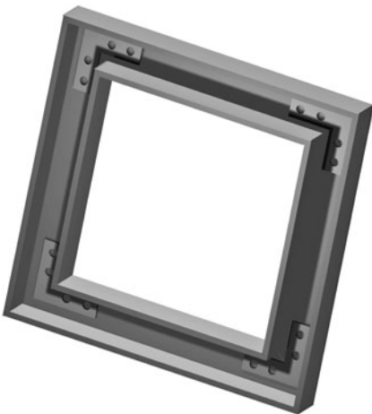
Figure 11-7 Solid metal frames can be constructed out of U-shaped aluminum channel, 3/8” wide L angle brackets, and metal fasteners. Cut the aluminum channel with a miter box and hacksaw.
