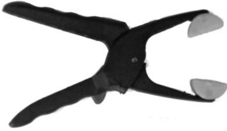
Figure 29-13 Small plastic tool clamp used in the tool clamp gripper.
