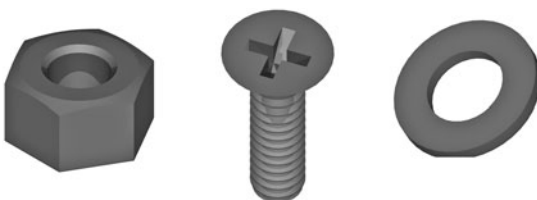
Figure 13-1 Nuts, screws, and washers are the fundamental pieces used in mechanical fastening. Nuts and screws are threaded to match; washer size is based on the diameter of the screw.
