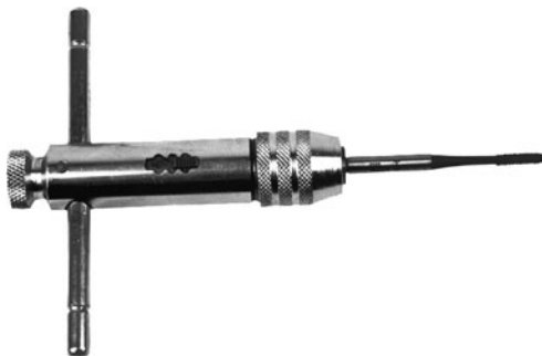
Figure 11-9 A T-wrench and tap are used to thread holes for mechanical fasteners. Be sure to drill the hole to the proper size for the tap you are using.
