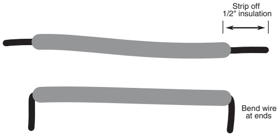
Figure 32-3 To make your own breadboard jumpers begin by stripping of 1/2" of insulation from both ends, being careful not to nick the wire (that weakens it and can cause the wire to break off easily). Finish by bending the wires at the ends.
