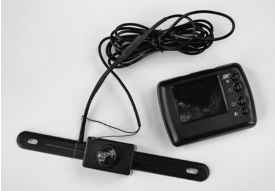
Figure 41-6 Backup camera system, designed to be mounted on the rear license plate holder of a car or van. The camera broadcasts color video to the receiver, which contains its own LCD screen.
