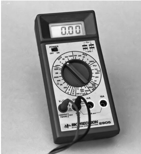
Figure 30-1 A digital multimeter checks resistance, voltage, and current. This model also performs simple checks of a number of common electronic components, including capacitors, diodes, and transistors.
