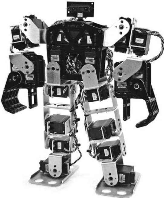
Figure 2-7 Bipedal (two-legged) robots present special challenges, not only in construction, but in programming. Standardized metal brackets, like those used here, make building easier by not requiring you to have a complete metalworking shop in your garage (though if you do, by all means use it!). (Photo courtesy Lynxmotion.)
