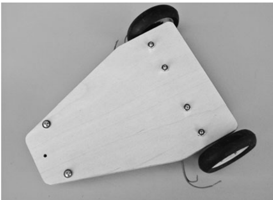
Figure 8-1 The PlyBot uses two Tamiya gear motors and wheels, plus a ball caster (or skid) for balance. It's made using a single piece of quarter-inch-thick 7" × 5" aircraft plywood.
