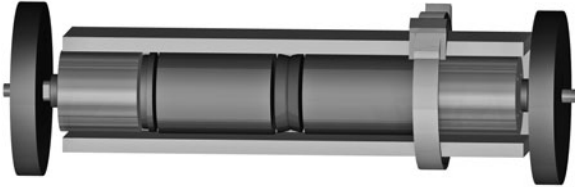
Figure 24-5 Motors in a differentially steered robot may be secured and aligned by placing them inside a strip of aluminum U-channel. The inside dimensions of the channel must be large enough to accommodate the girth of the motor. Use plastic cable-ties to hold the motors in place.
