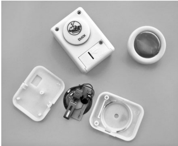
Figure 46-1 An assortment of sound modules with prerecorded sounds and songs on them. Most modules can be hacked to operate from electronic control.
