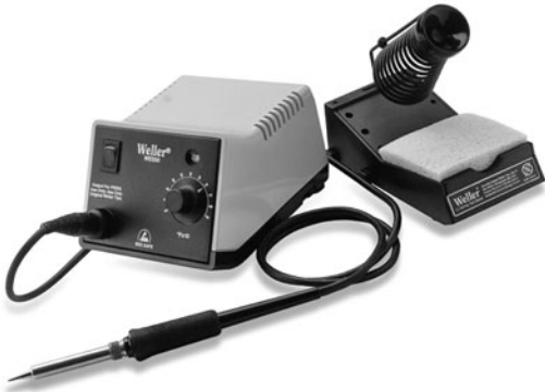
Figure 30-4 Soldering station with adjustable heat output. This model does not have a temperature indicator, but you can infer it by adjusting the output to where it just begins to melt solder. Remember that different compositions of solder have different melting points. (Photo courtesy Cooper Tools)
