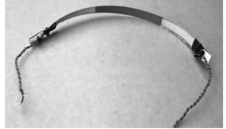
Figure 42-19 Prototype piezo film bend sensor. Two short pieces of piezo film are taped to a thin plastic sheet (a school report cover); the sheet acts as a backing and is formed into a half-circle to detect when the robot bumps into something.
