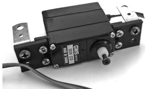
Figure 24-7 A pair of servo mounting tabs, shown with servo and 3/8" metal angle brackets for securing to a robot base.
