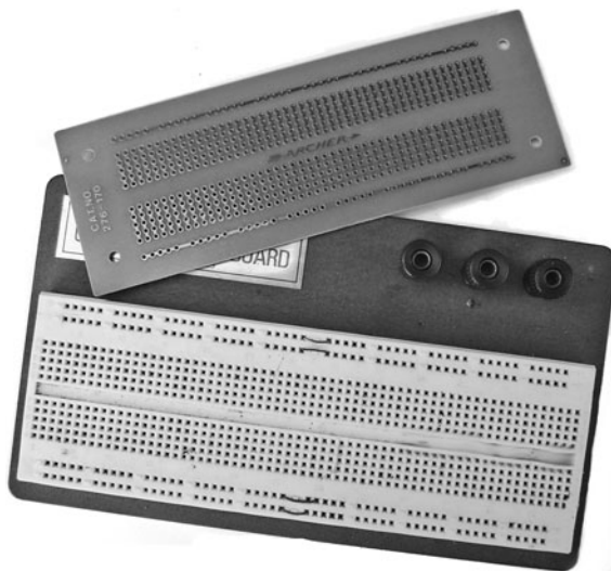
Figure 33-1 A solderless breadboard and a companion solderboard. Test your circuits on the solderless breadboard, and once the design is finished, debugged, and working, transfer the components to the solderboard following the same arrangement.
