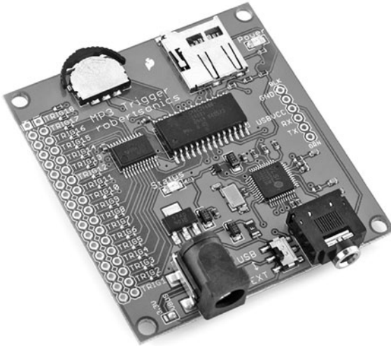
Figure 46-7 All-in-one MP3 playback board, which can be connected to a switch or a microcontroller for fully automated sound clip selection. It supports up to 256 sound clips, stored on a \mu SD card. You can use your PC to copy sound files to the card. (Photo courtesy SparkFun Electronics.)
