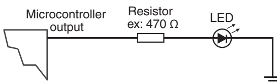
Figure 40-9 Some electronic devices, such as light-emitting diodes, require current limiting, or else damage to the circuit could result. The resistor reduces current to the LED.
