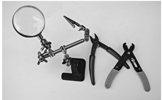
Figure 30-5 Trio of the most used tools for working with electronics: a vise or “third hand” (magnifier optional, but handy), flush wire cutters, and wire strippers.
