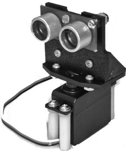
Figure 23-10 A servo used to rotate a sensor, mounted on a bracket.
