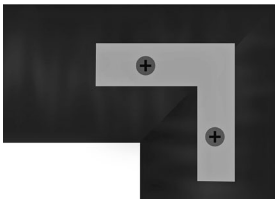
Figure 7-10 An L angle bracket connects the frame pieces together. Use machine screws, nuts, and washers for a solid construction.
