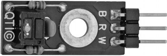
Figure 43-3 Integrated IR emitter and detector modules provide a quick way to add light sensors to your robot. Standard .100" connector pins provide easy hookup. (Photo courtesy Parallax Inc.)
