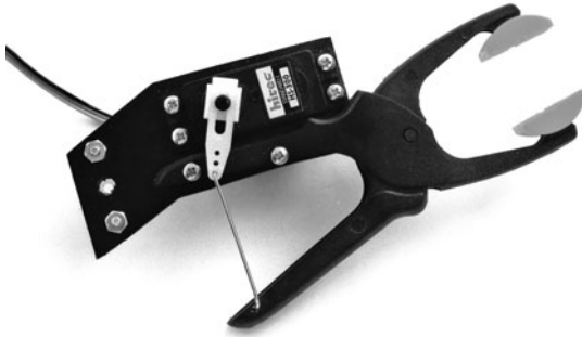
Figure 29-17 Finished tool clamp gripper, showing the activating rod between the clamp and the R/C servo motor.
