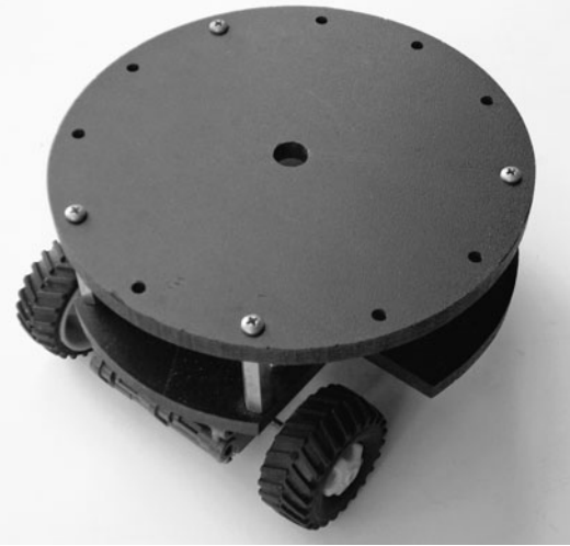
Figure 26-5 The BasicBot uses one or two decks, a Tamiya Twin Motor gearbox kit, a set of small tires, and a ball caster for balance. Construction takes less than an hour.
