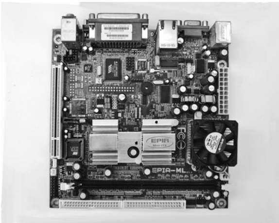
Figure 34-3 Mini-ITX motherboard, able to run Windows, Linux, and many other modern operating systems. Its small size and miserly power requirements make the board a perfect contender for use in a medium- to large-size robot.
