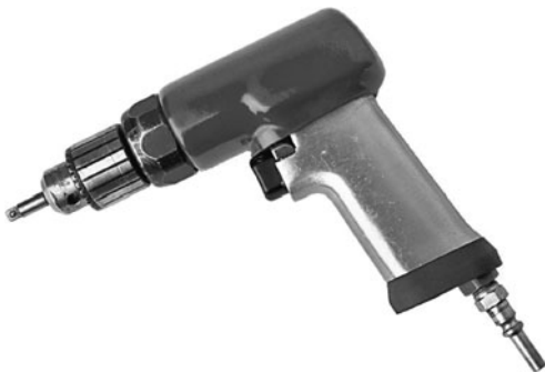
Figure 6-5 A pneumatic drill is lighter and smaller than an electric drill, but it needs a constant source of compressed air.
