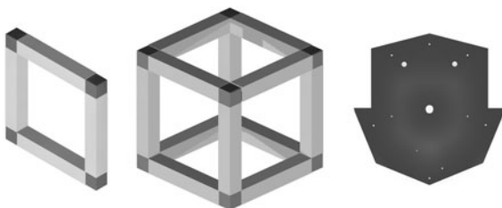
Figure 5-2 The three basic types of robot bases: square frame (it can actually be made of wood, plastic, or metal), a box frame, and a shaped base that provides the structure for the robot's components.
