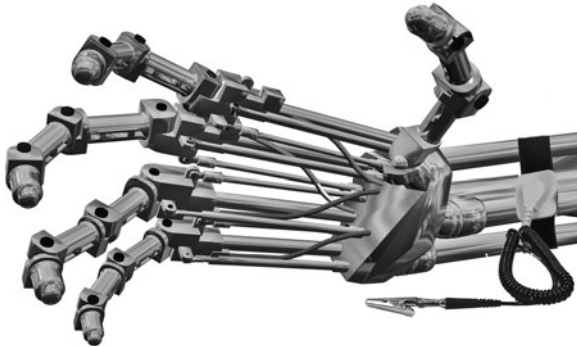
Figure 4-1 An antistatic wrist strap draws static electricity from your body, helping to prevent damage to sensitive electronic components. Be sure to use the wrist strap according to the manufacturer's instructions.
