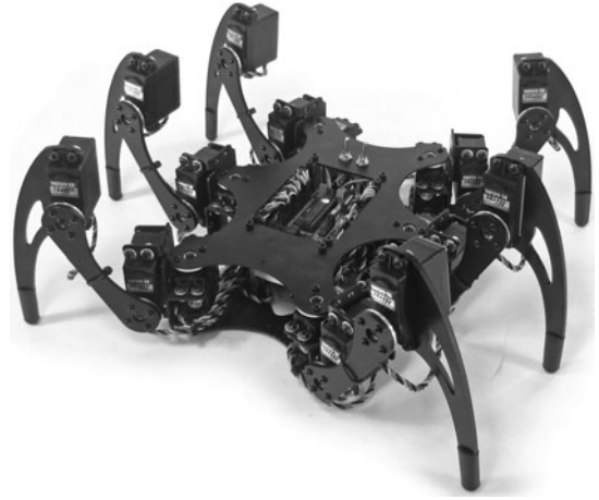
Figure 2-6 A rewarding project is a multilegged walking robot, such as this model that has six legs. It's operated using three individual motors per leg, for a total of 18 motors. (Photo courtesy Lynxmotion.)
