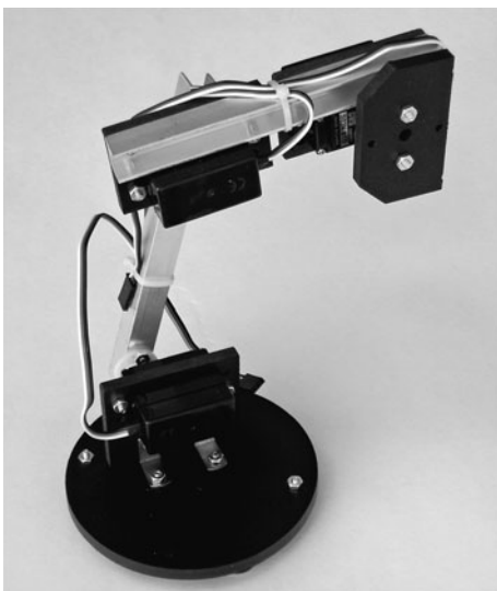
Figure 28-7 Completed robotic revolute coordinate arm. Attach the arm to a base or robot and add a gripper mechanism.
