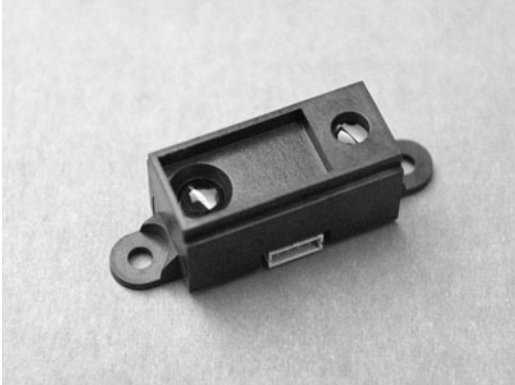
Figure 43-9 Example Sharp IR sensor. This variation of the sensor has convenient screw eyelets for easy mounting.
