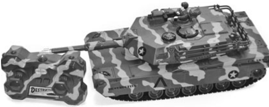
Figure 16-6 A store-bought tank toy contains motors, rubber tracks, drive sprockets, and idler wheels—all can be repurposed for a desktop tracked robot.
