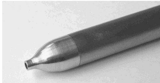
Fig. 8 The view of the designed flow nozzle
