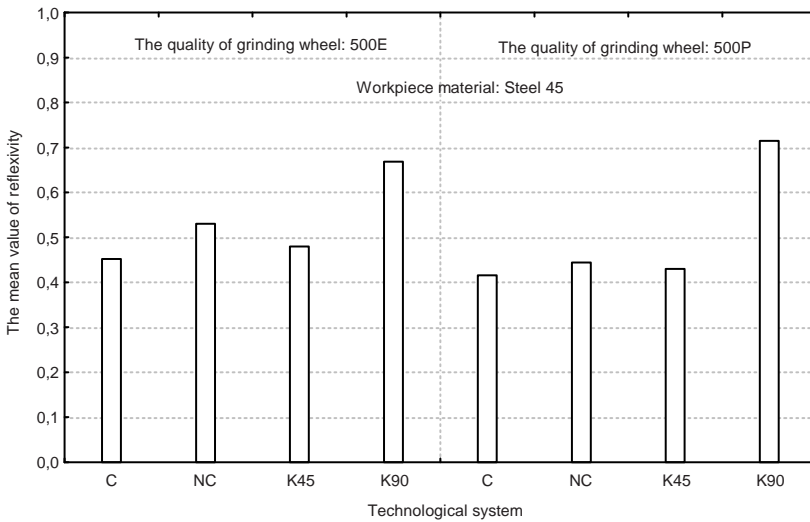
Fig. 4. The influence of technological system on the mean value of reflexivity steel 45 surface which was polishing the grinding wheels 500E and 500P of polyurethane bond
