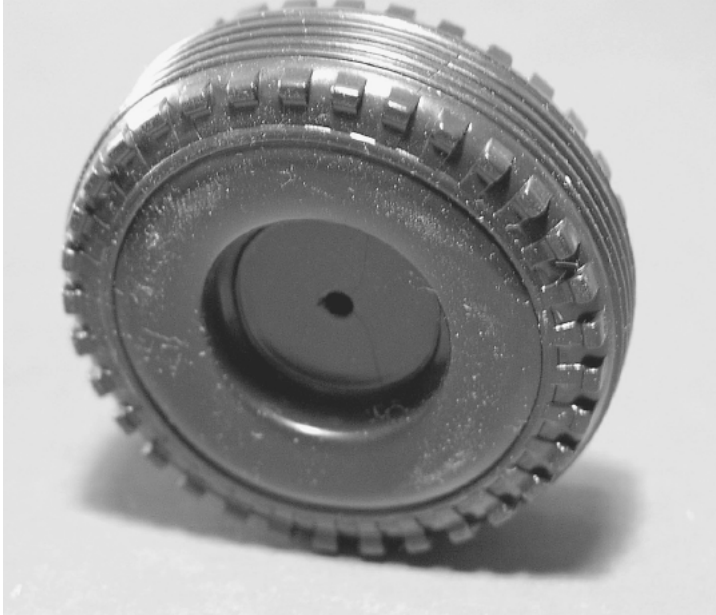
Figure 9.12 Rubber wheel used to friction fit onto gearbox motor shaft.
