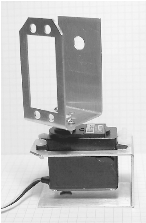
Figure 12.22 Assembled bottom brackets for robotic arm.
