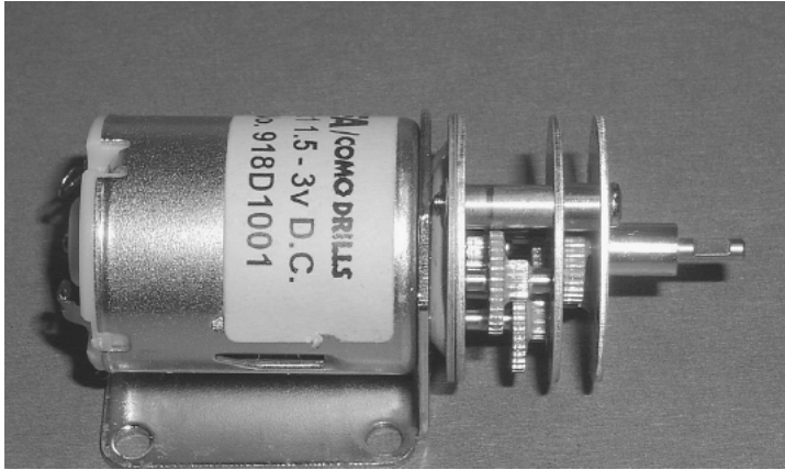
Figure 9.10 Gearbox motor showing cutaway on output shaft.
