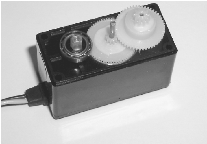
Figure 8.7 Top view of servomotor gears with plastic clip removed.
