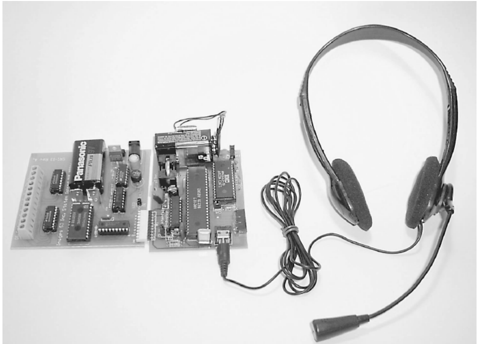
Figure 11.12 SRI-03 connected to speech recognition circuit.
