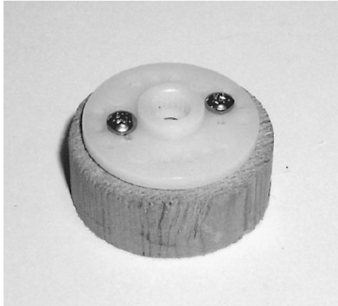
Figure 12.42 A 1-in \times 0.40-in wood dowel with round servomotor horn.
