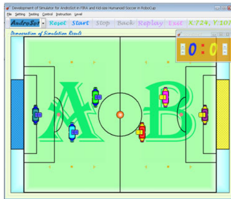
Fig. 2. The interface of the simulator, which includes the game field, the main menu and the scoreboard
