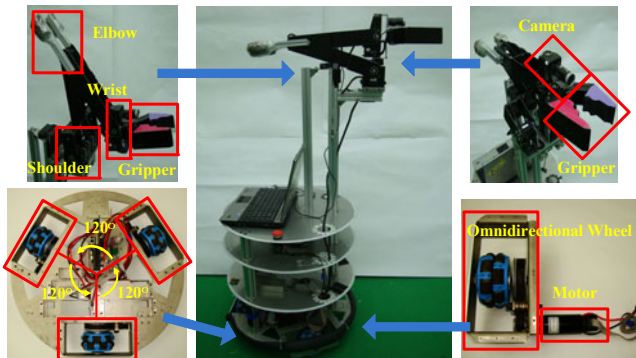
Fig. 2. Pictures of the implemented robot and their description
