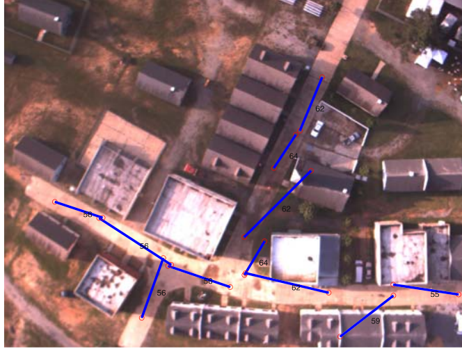
Figure 5. Preliminary experimental radio connectivity map for the MOUT site obtained using our multi-robot testbed.
