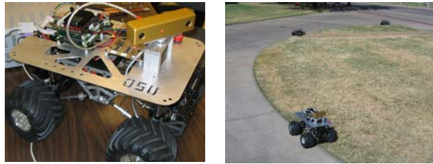
Figure 1. (a) MARHES multi-vehicle experimental testbed, and (b) setup for perimeter detection.
