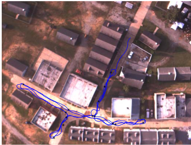
Figure 2. Trajectory of a robot navigating using a sequence of waypoints. The waypoints are depicted as '*' and the robot executes the sequence twice.
