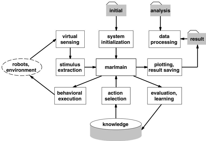
FIGURE 14.1. The architecture of the multi-agent reinforcement learning toolbox.
