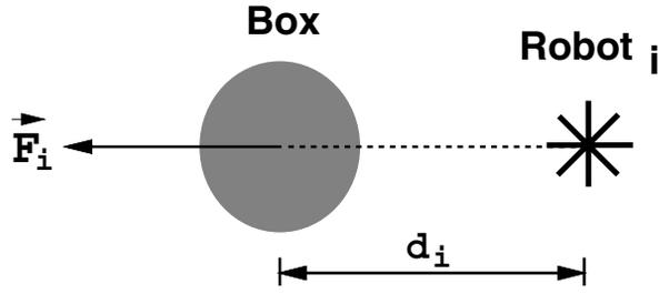
FIGURE 11.3. A top view of collective box-pushing (Note: for the sake of clarity, only one robot is depicted) where group robots, marked with \*, move toward a box, signified by a shaded area. When their distances  $d_i$  are less than or equal to threshold  $l_0$ , pushing forces will be exerted on the box by the robots, according to the model of a repulsive pushing force (refer to the text).
