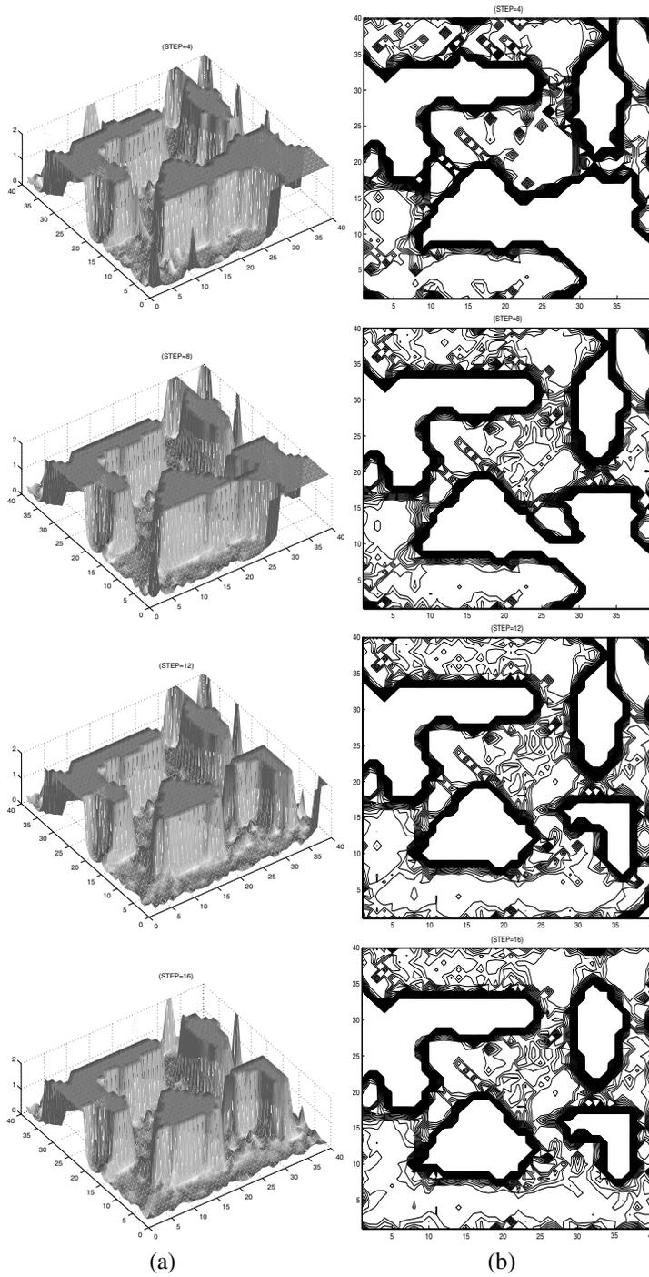
FIGURE 12.8. (a) The snapshots of a potential field map at four different time steps, as built by a group of decentralized robots with the motion selection mechanism of *Directional2*. (b) The corresponding contour plots.
