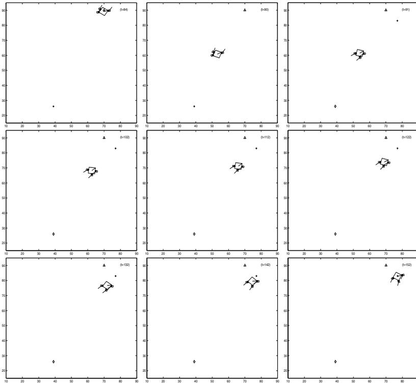
FIGURE 11.28. The snapshots of collective cubic box-pushing in which a new goal location, denoted by +, is set at generation 91, before an old one, denoted by  $\diamond$ , is reached. Like the preceding experiment, the robots again successfully readapt their collective movements. The process of collective pushing before generation 84 has been shown in [Figures 11.19](#) and [11.20](#).
