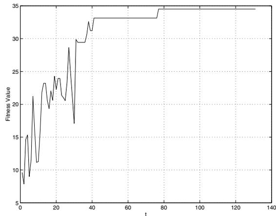
FIGURE 11.27. A fitness function plot corresponding to the movement selection and readaptation of three group robots, as shown in [Figure 11.26](#), over the entire evolution process of 131 generations.
