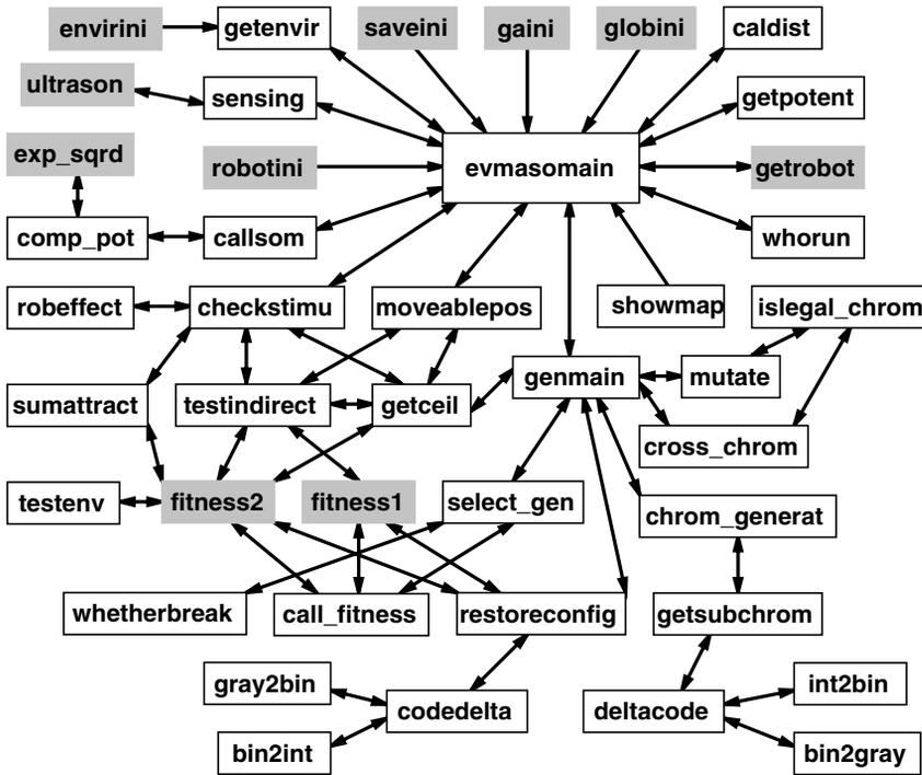
FIGURE 14.20. The calling tree for the evolutionary self-organization toolbox.
