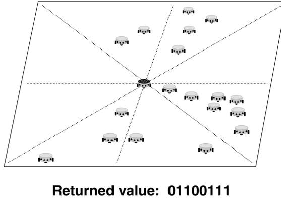
FIGURE 6.4. A schematic diagram illustrating long-range sensors.
