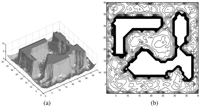
FIGURE 13.8. *Non-evolutionary mode*: (a) A potential field map built by 6 robots with predefined reactive motion strategies after 24 movement steps. (b) A contour plot for the obtained potential field map (© 1999 IEEE).
