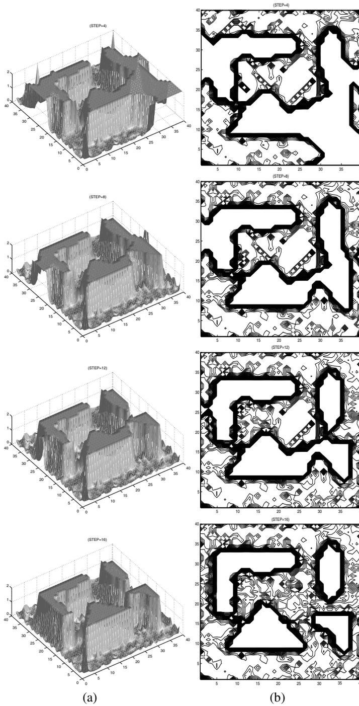
FIGURE 12.7. (a) The snapshots of a potential field map at four different time steps, as built by a group of decentralized robots with the motion selection mechanism of *Directional1*. (b) The corresponding contour plots.
