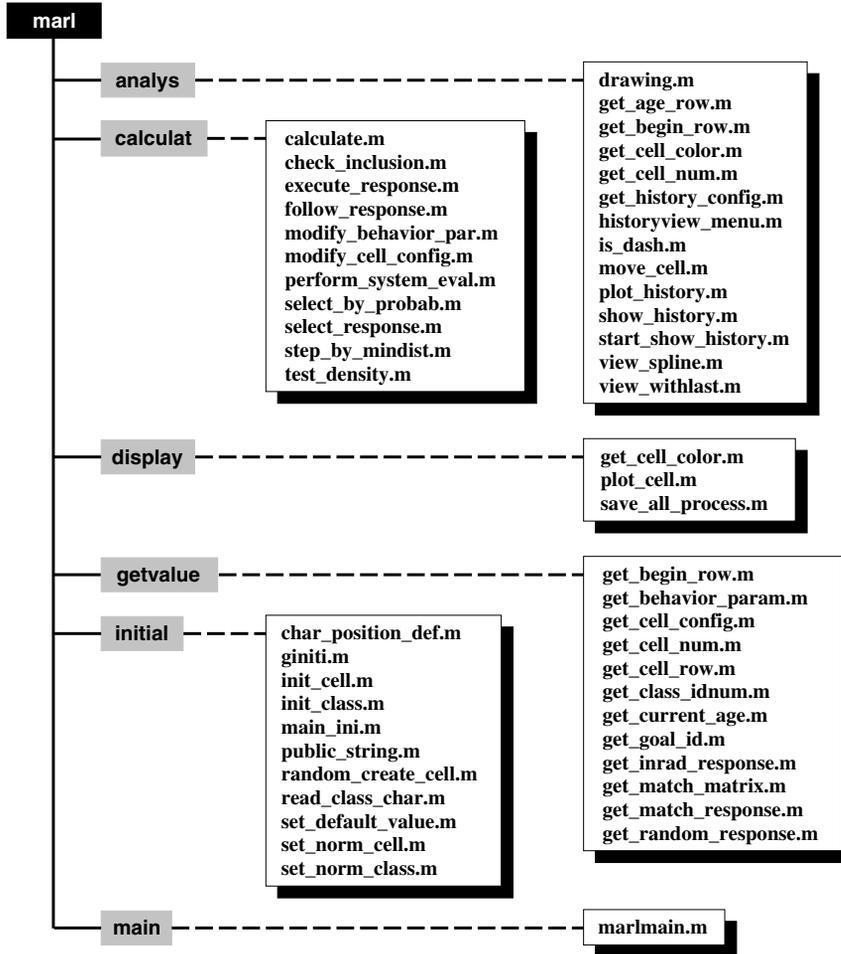
FIGURE 14.2. The file structure for the multi-agent reinforcement learning toolbox.
