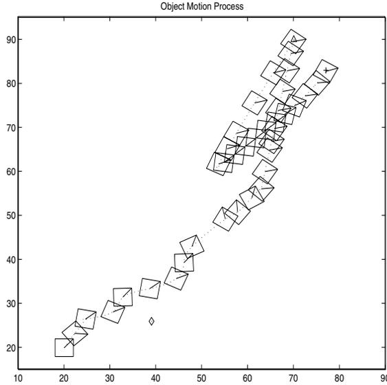
FIGURE 11.29. The trajectory of a cubic box collectively pushed by three group robots. In this case, a new goal location, denoted by +, is set before an old one, denoted by  $\diamond$ , is reached. The successful readaptation of the robots is reflected in the smoothness of the observed trajectory. In the trace, the diagonal inside the cubic box signifies the orientation of the box.
