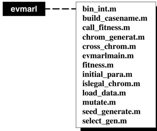
FIGURE 14.5. The file structure for the evolutionary multi-agent reinforcement learning toolbox.
