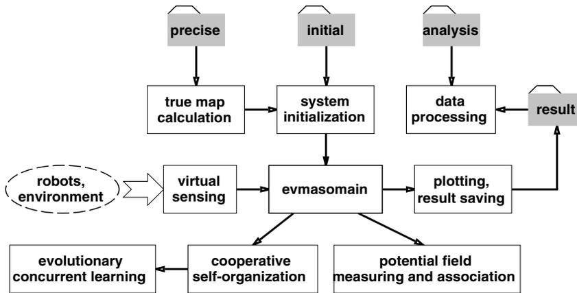
FIGURE 14.18. The architecture of the evolutionary self-organization toolbox.
