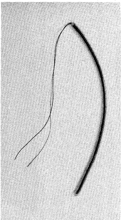
Figure 5.24. The Rubbery Ruler provides a unique way to measure deformations and relative positions.
