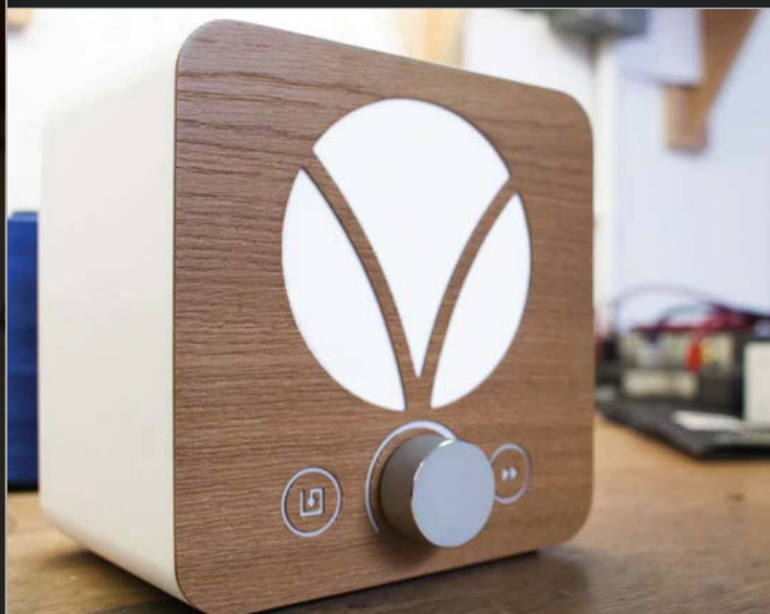
Above Capacitive touch sensors are used for the ‘skip’ and ‘save’ buttons
