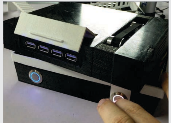
Above The flap is motorised, revealing the USB ports when turned on, thanks to a custom Python script
