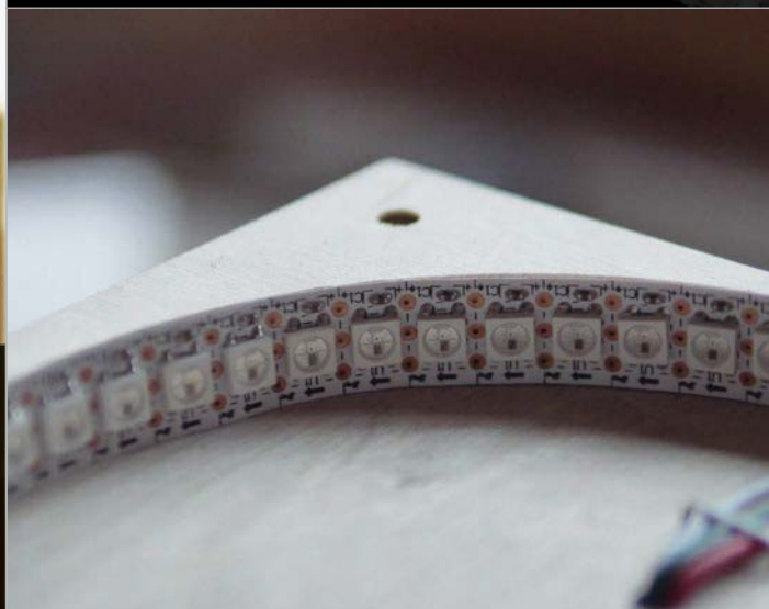
Above A ring of NeoPixels is used to create the geographically controlled light effect
