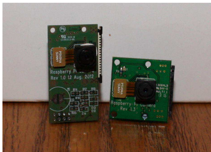
Prototype camera board (left) and final camera board (right)
