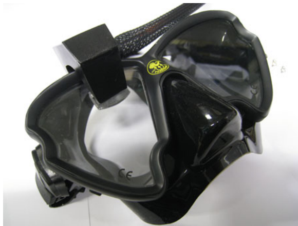
Fig. 3.6 Innovative graphical head up display mounted on a commercial diving mask
