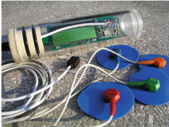
Fig. 4.7 First prototype in a Lexan housing
