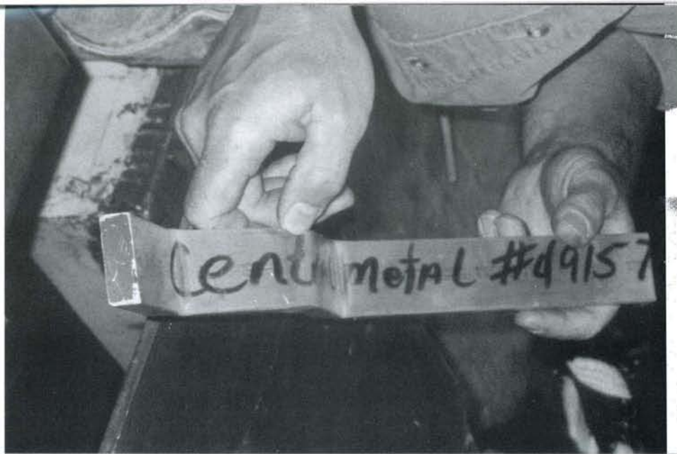
This one-inch bar of 6061 aluminum was used to make test bends. The test was successful, meaning it was safe to use this alloy on the actual project under construction.
